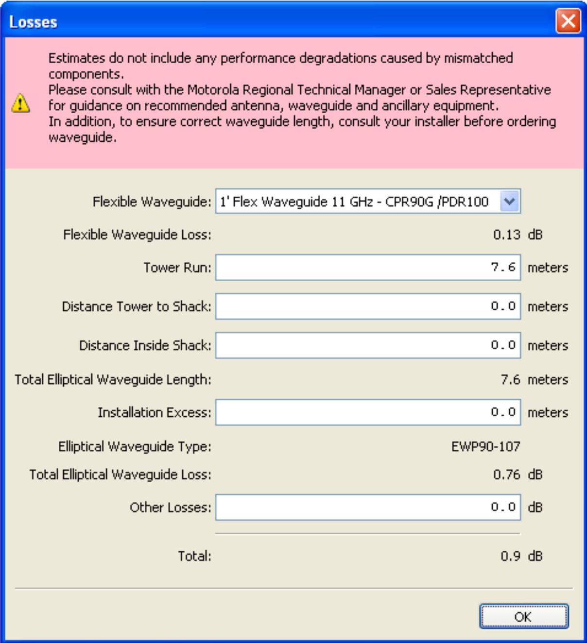
Figure 3.61: Losses (Long Waveguide)
