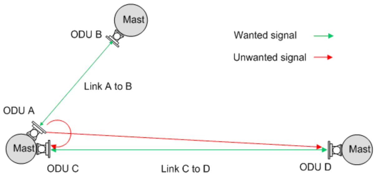
Figure 4.6: Interference Between ODUs
