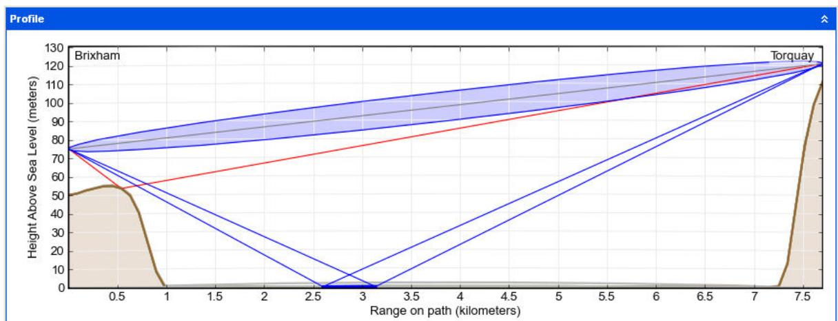
Figure 3.73: Profile with Reflection Visible
