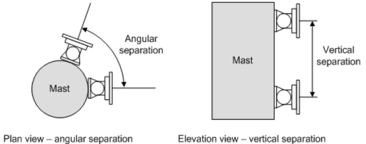
Figure 4.7: Separation of PTP 600 Units on a Mast
