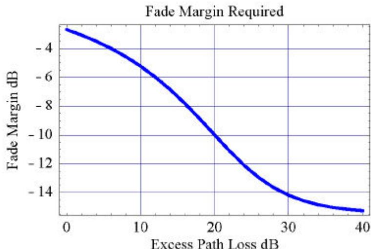
Figure 4.2: Fade Margin vs Excess Path Loss for 99.99% Link Availability
