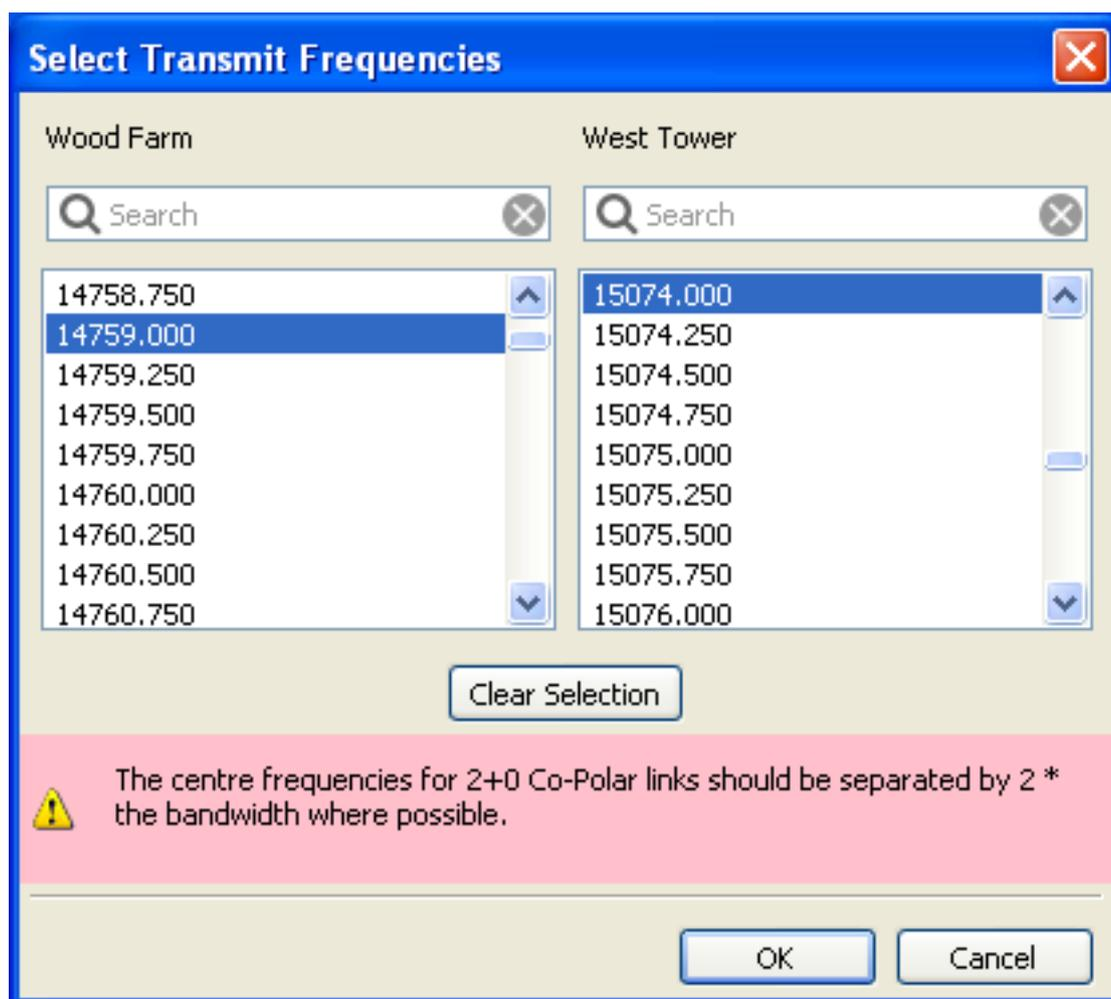
Figure 3.58: Select Transmit Frequency 2+0 Co-Polar Adjacent Channel Error
