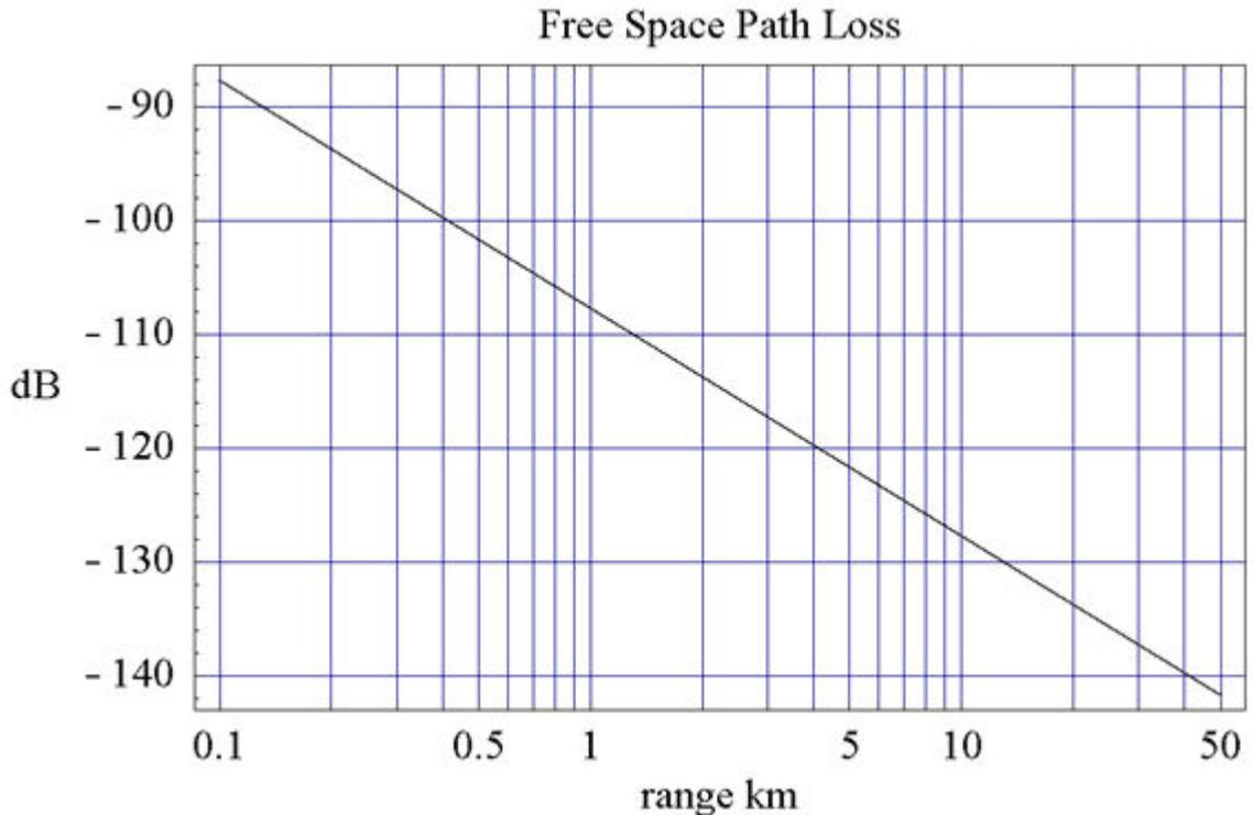
Figure 4.1: Free Space Path Loss at 5.8 GHz
