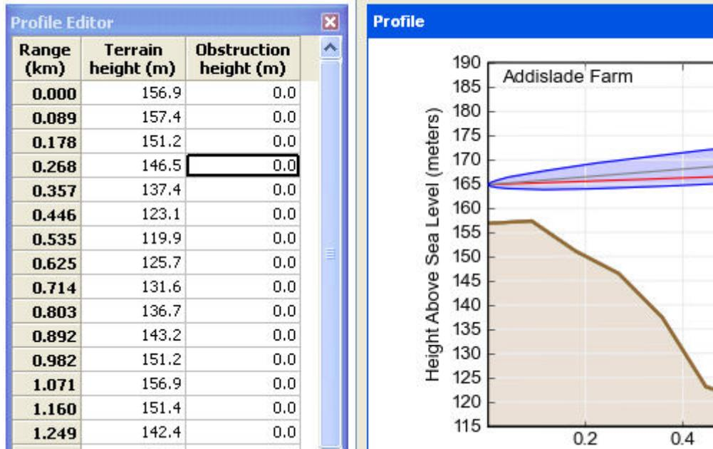
Figure 3.77: Unadjusted profile near antenna site
