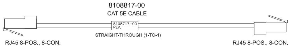
IDU to PSU 100BaseT & 10BT to Hub
