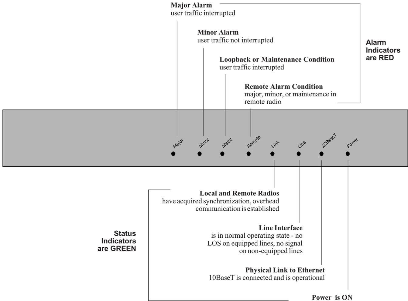
On a power-up cycle all LEDs turn on and then go off in the following sequence: 10BaseT, Line, Link, Remote, Maint, Minor, Major, as the boot code runs through its start up stages.
