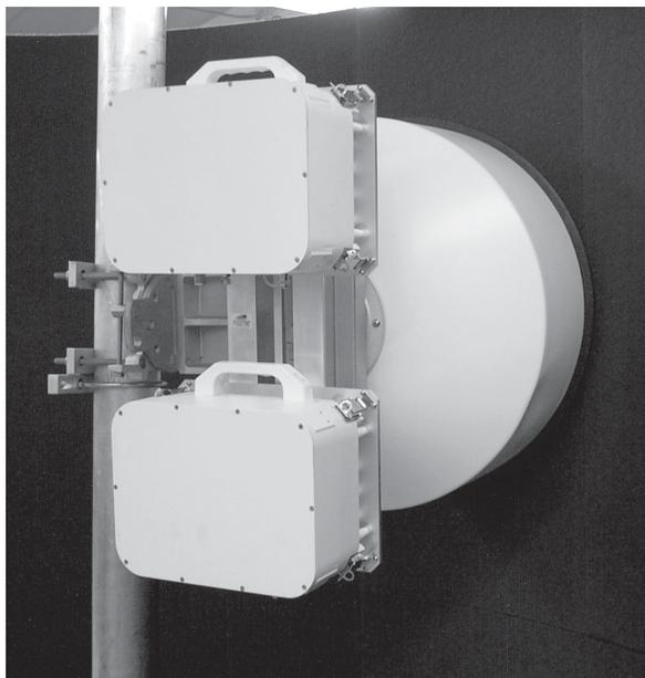
5. The above procedure will provide vertical polarization for the antenna. A horizontally polarized coupler/mounting assembly is available for special order. Contact MNI.
