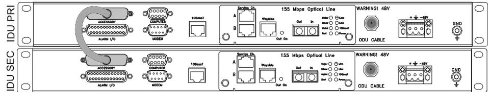
External switching, serial data protection mode lets customers protect payload using their own add-drop multiplexers. The Protection Switch unit is not used. A special cable assembly, Figure 4, connects the accessory ports of the IDUs. IDU logic selects active path.
