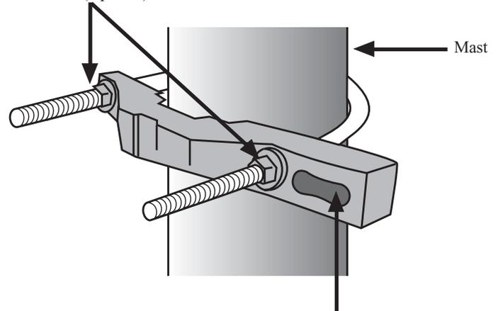
Note: Location of Azimuth adjustment hole
