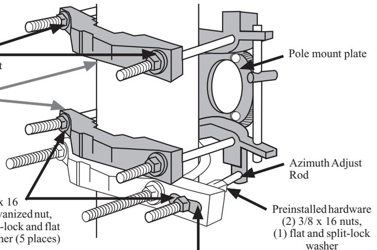
**Note:** Hand tighten nuts to allow for adjustment. Torque to spec. after alignment.
