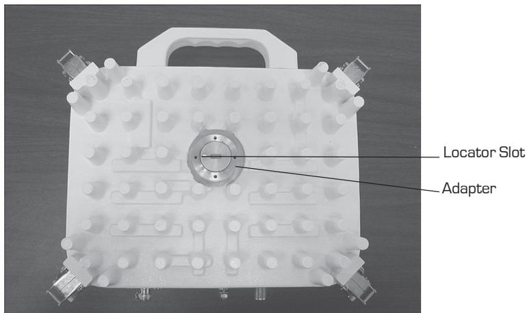
4. Attach the RF units with adapter to the coupler assembly. Align RF units to the center feed on the coupler. Carefully push the assemblies together. Orient the RF unit handle up. Latch the RF units to the coupler using the four chassis clamps. Figure 12 shows the completed assembly.
