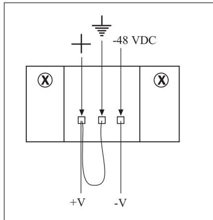
When a -48 VDC supply (positive ground) supply is used, wire the mating power connector to the prime power source shown here.
