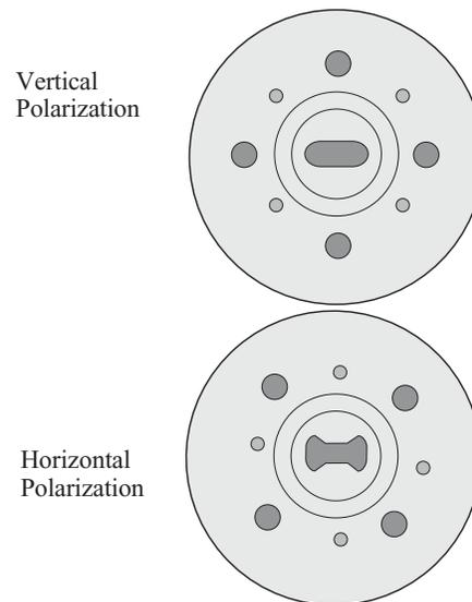
3. If an antenna transition has to be changed from vertical to horizontal, follow the procedure below:
