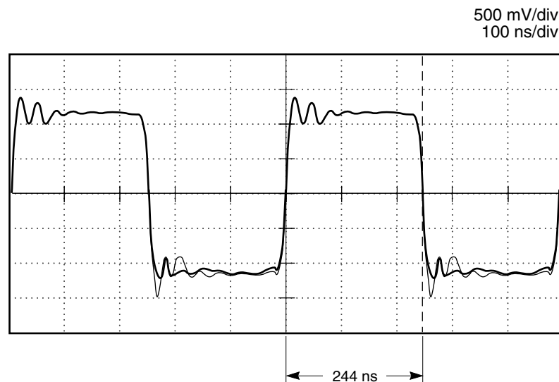
Figure E2-5. 2048 kHz Pulse Width Test
