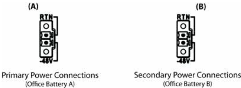
Figure 2-14. Power and Ground Connections on the TimeProvider 5000
