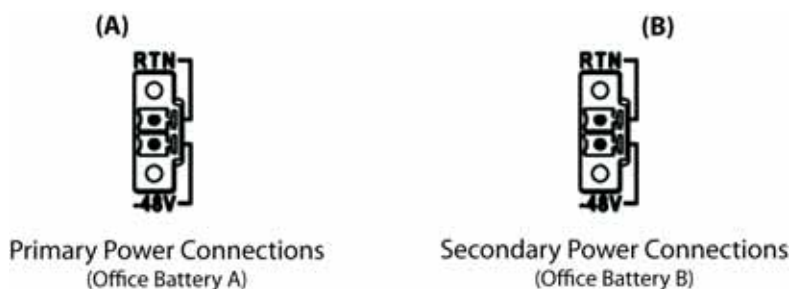
Figure 2-34. Power and Ground Connections on the TimeProvider 5000
