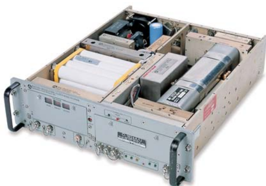
Shows Replacement Caesium Beam Tube installation in FEI instrument.
