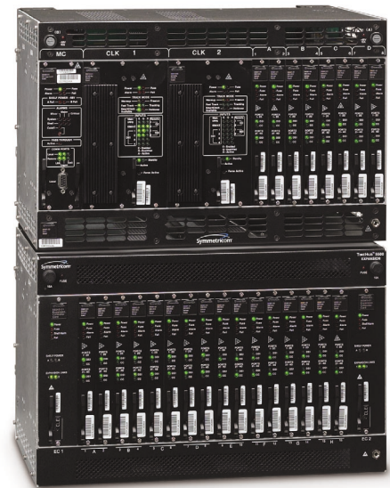
FIG.1 TimeHub 5500 with Expansion Shelf
