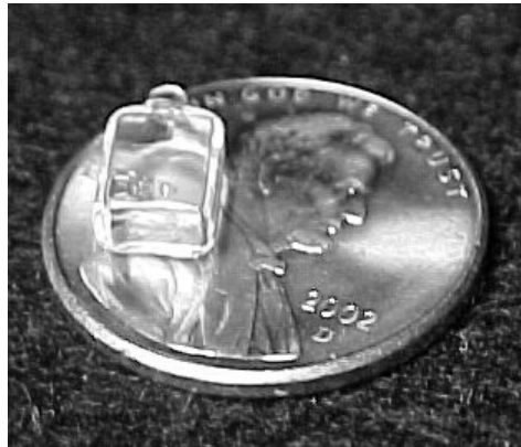
Figure 6: Resonance cell containing cesium and buffer gas mixture
