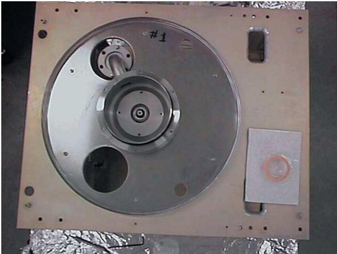
Top View of Source Chamber, Collimator, and Dissociator
