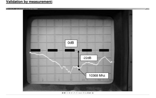
10mm thick shim measured by F1JRZ, return loss not far from the simulation. Reflections in the measurement room are visible, we also see that the shim is clearly too long.
