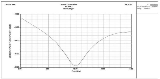
Of course, since the impedance transformer is a narrowband device, the matching range is reduced. Matching -21.5dB at 10368Mhz. Quite acceptable, if confirmed on the actual horn. The length seems to be reworked (shorten).
