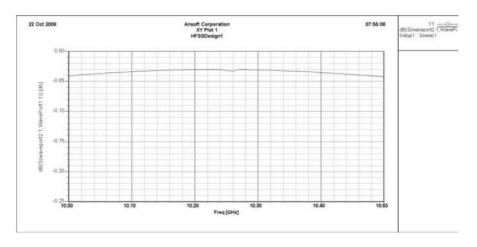
Losses are minimal (note the 2 adapter access guides are included), less than 0.1db in simulation (probably a little more in reality)
