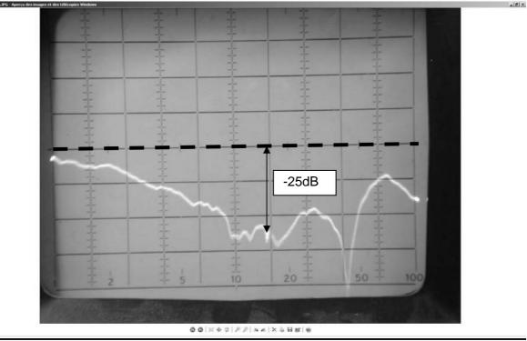
The improvement is confirmed. However, the adaptation is less good than the simulated value. This question should be investigated further, for example by characterizing the directivity of the measurement coupler, and the influence of reflections caused by the horn's environment. There is also the influence of the coaxial adapters used for the measurement. The reason for the "dip" at -45dB (11.2Ghz) is unknown and not reproducible on the simulator. Is it due to the measurement?
