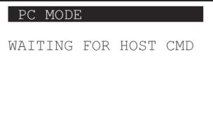
To command T101 to tune to a specific frequency, the host program shall transmit a six-digit frequency in ASCII characters via the serial port.
