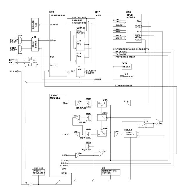
Figure 6-1 Logic Board Block Diagram
