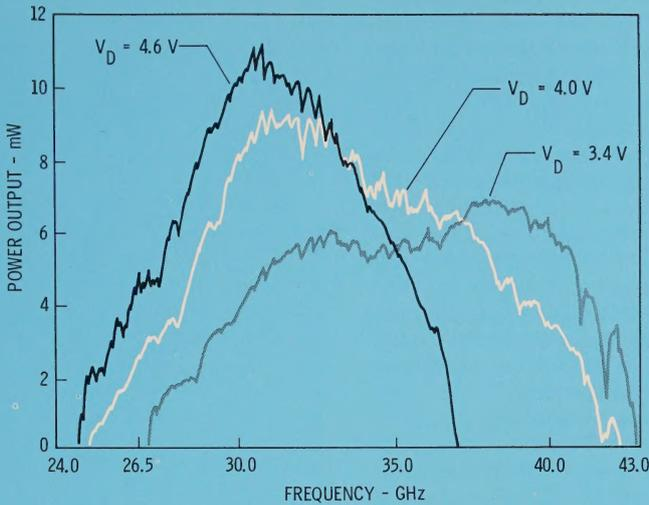
Fig. 3. Power Output of a YIG-tuned GaAs Oscillator (WJ-5610-1) for diode bias voltages at 3.4, 4.0 and 4.6 volts.
