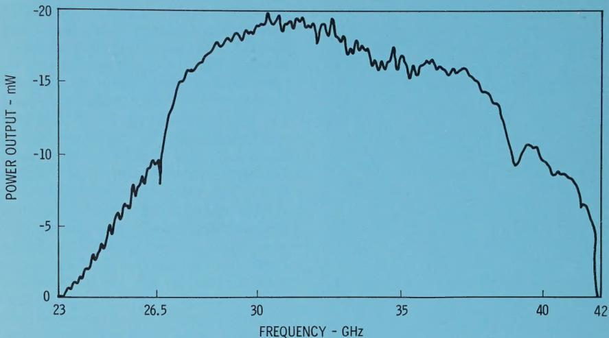
Fig. 7. Power Output of a Ka-band Oscillator with Diode E-Field parallel to the Magnetic Field. The Curve is obtained by programming the diode bias from 3.5 volts to 4.6 volts.
