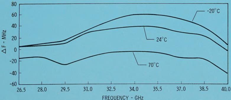
Fig. 4. Frequency Accuracy of a Ka-band Oscillator for baseplate temperatures at -20°C, 24°C and 70°C.
