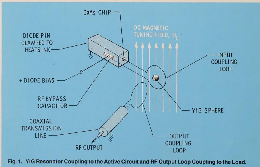
Fig. 1. YIG Resonator Coupling to the Active Circuit and RF Output Loop Coupling to the Load.
