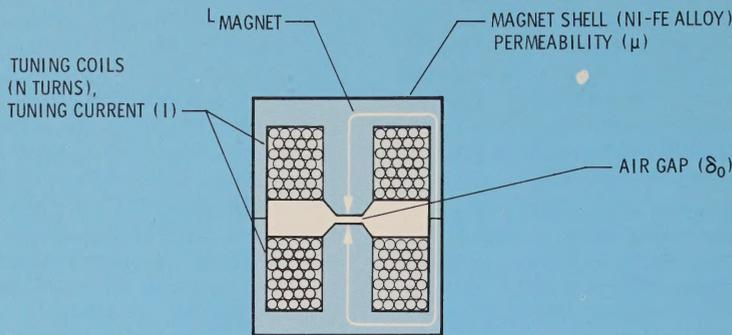
$$\text{FIELD IN AIR GAP: } H_0 \text{ (GAUSS)} = \frac{0.4 \pi N I \text{ (A)}}{\delta' \text{ (cm)}}$$
