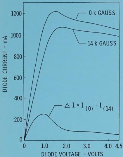
Fig. 5. Diode dc characteristics with and without Magnetic Field and Diode E-Field orthogonal to the Magnetic Field.
