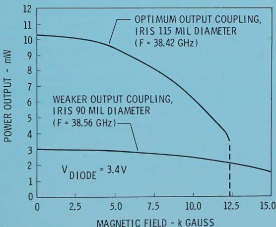
Fig. 6. Power Output to the Test Cavity Oscillator in a magnetic field and Diode E-Field orthogonal to the Magnetic Field.
