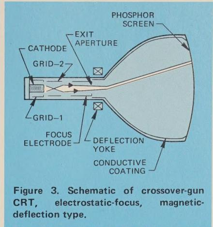
**Figure 3. Schematic of crossover-gun CRT, electrostatic-focus, magnetic-deflection type.**
