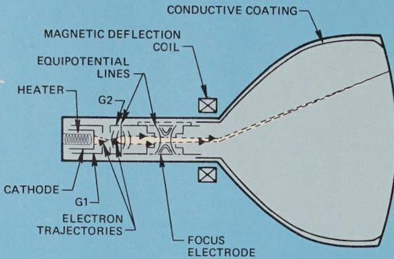
Figure 11. Unipotential electrostatic-focus gun.
