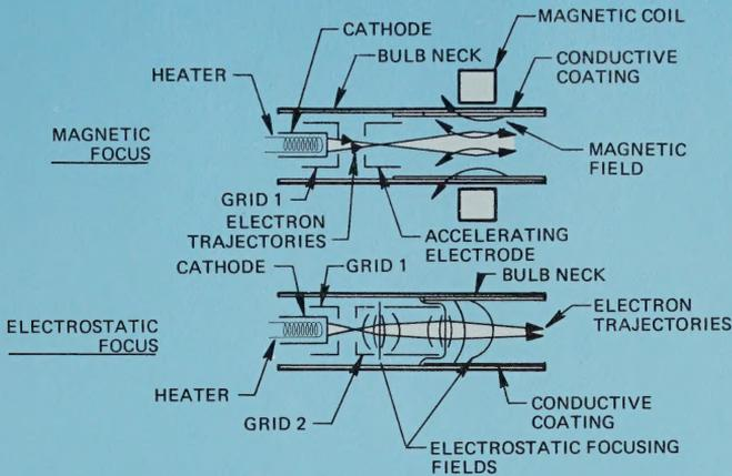
Figure 9. Comparison of electrostatic and magnetic focusing.
