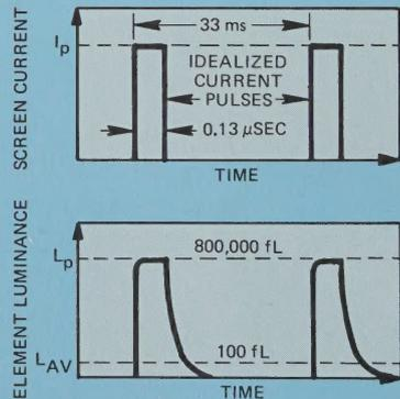
Figure 1. Current and luminance for a single CRT resolution element of a 500-line TV raster.
