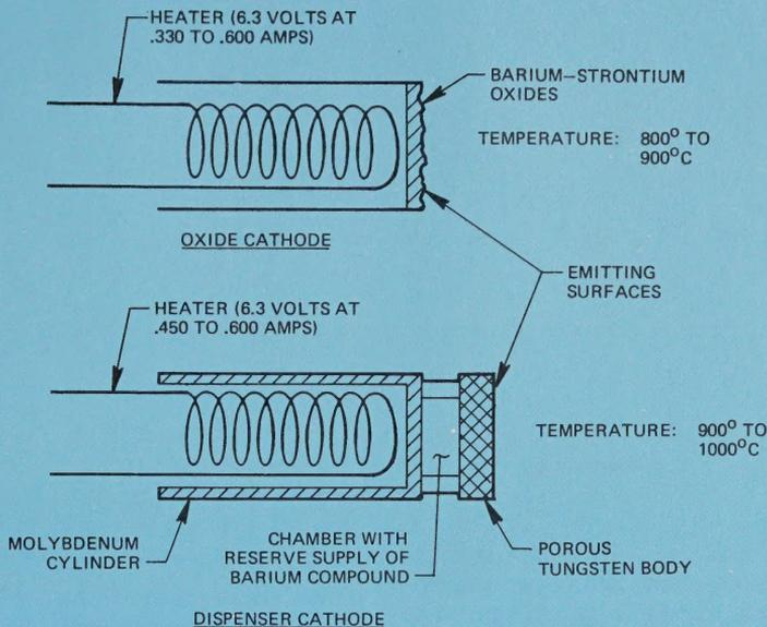
Figure 6. Comparison of oxide and dispenser cathode structures.
