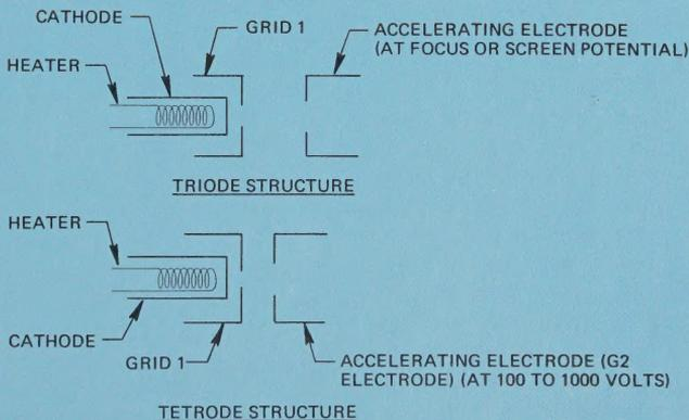
Figure 7. Comparison of triode and tetrode structures.
