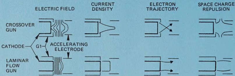
Figure 8. Comparison of crossover and Laminar-flow beam formation.
