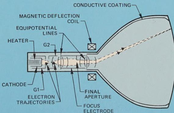
Figure 10. Bipotential electrostatic-focus gun.
