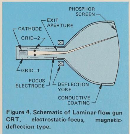
**Figure 4. Schematic of Laminar-flow gun CRT, electrostatic-focus, magnetic-deflection type.**
