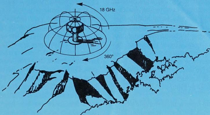
HORIZONTAL ANGLE PORTRAYS AZIMUTH COVERAGE.
