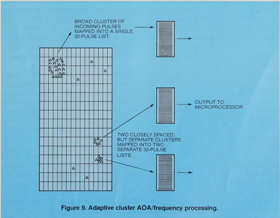
Figure 9. Adaptive cluster AOA/frequency processing.
