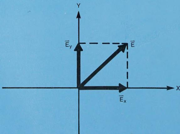
Figure 3. Decomposition of electric-field vector into orthogonal components.
