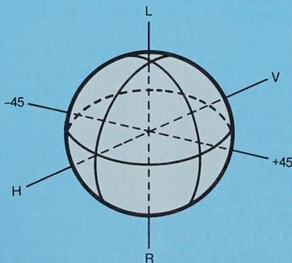
Figure 6. The Poincaré Sphere.
