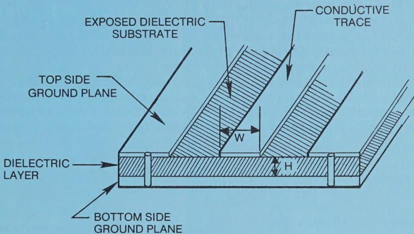
Figure 2. Printed-wiring board description.
