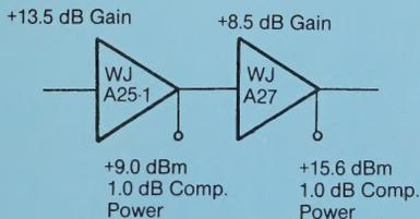
**Figure 9. Two-stage amplifier cascade.**
