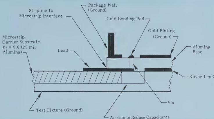
**Figure 9. A cross-sectional view of the interface between the test fixture and the surface-mount package.**
