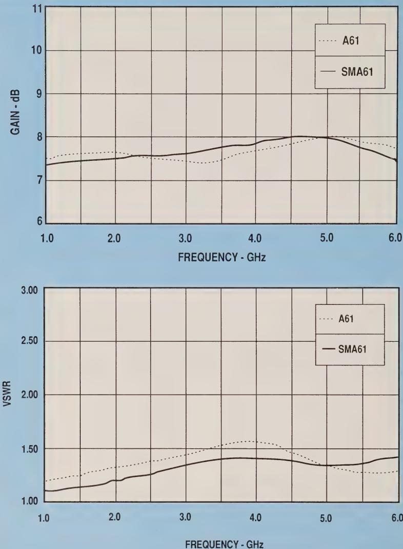
**Figure 10. Electrical performance comparison of the A61 amplifier in TO-8 and SMA61 packages.**
