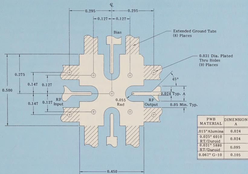
Figure 5A. Printed-wiring-board layout for the SMTO-8: 9-hole configuration.
