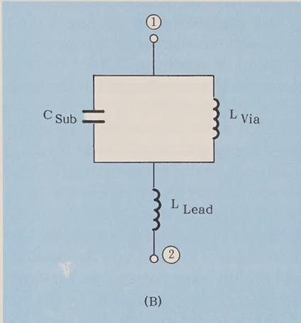
**Figure 3B.** An electrical model of the metal via, ceramic base and kovar lead-frame.
