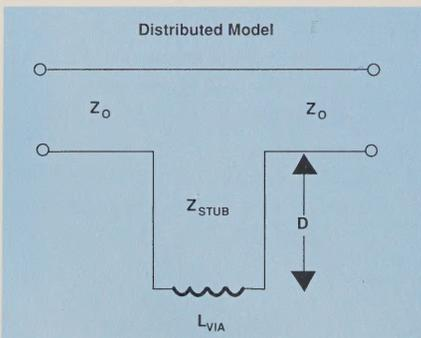
**Figure 4.** An electrical model of the surface-mount packages using distributed elements. The length,  $D$ , is the distance between the center of the lead and the closest ground via.
