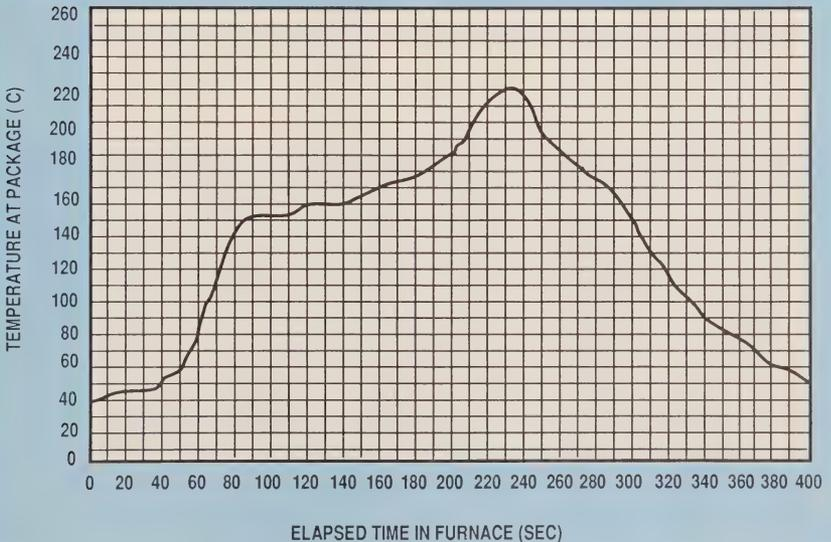
**Figure 12. The temperature profile used to reflow the solder during package mounting.**
