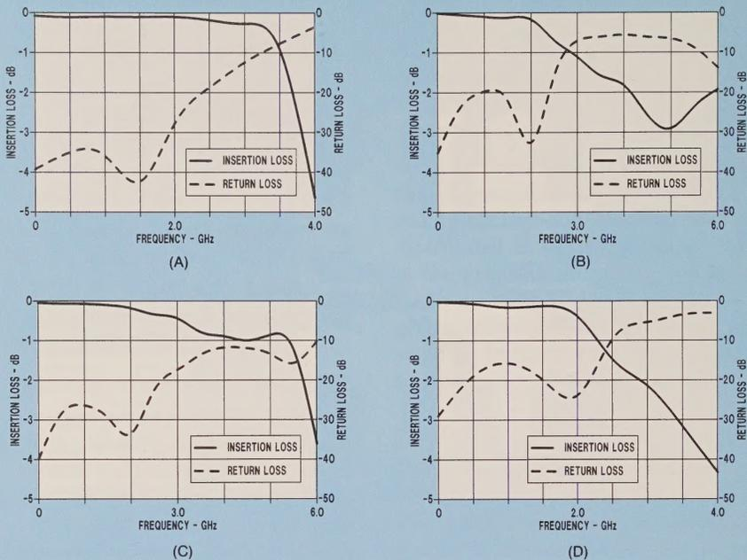
**Figure 8. Insertion loss and return loss of the SMT0-8 package mounted with the 4-hole configuration on: A) 0.062" G10, B) 0.025" 6010 RT/Duroid®, C) 0.031" 5880 RT/Duroid®, and D) 0.015" 96% alumina.**
