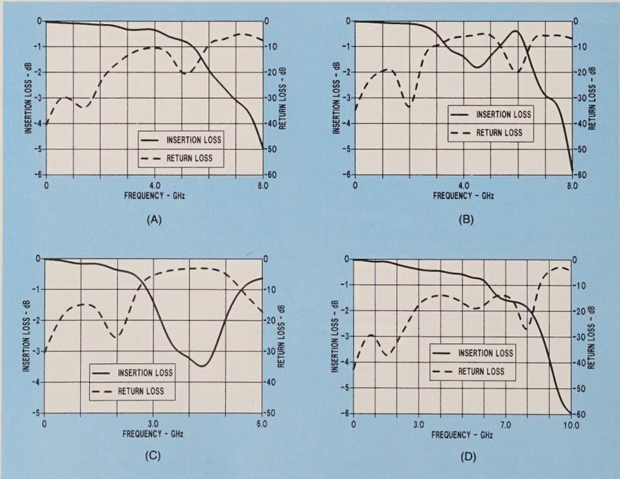
**Figure 6. Insertion loss and return loss of the SMT0-8 package mounted with the 9-hole configuration on: A) 0.062" G10, B) 0.025" 6010 RT/Duroid®, C) 0.031" 5880 RT/Duroid® and D) 0.015" 96% alumina.**
