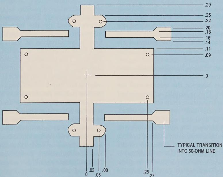
Figure 7B. Printed-wiring-board layout for the SMFLAT: 8-hole configuration.
