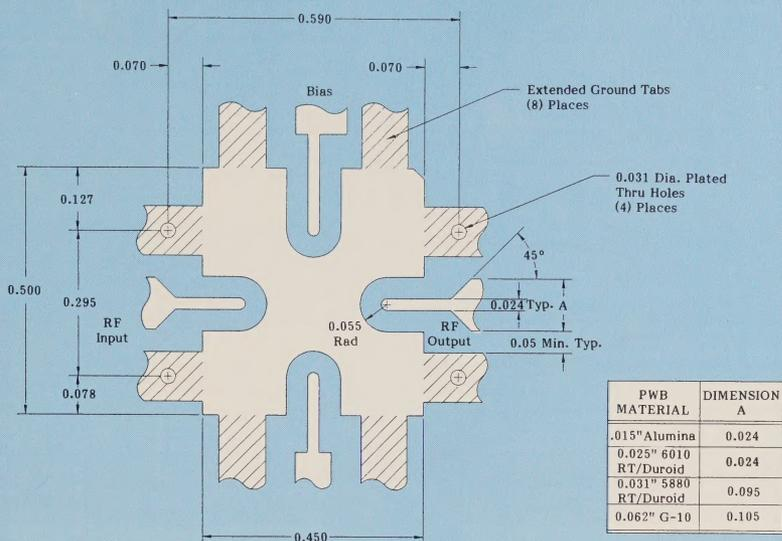
Figure 7A. Printed-wiring-board layout for the SMTO-8: 4-hole configuration.
