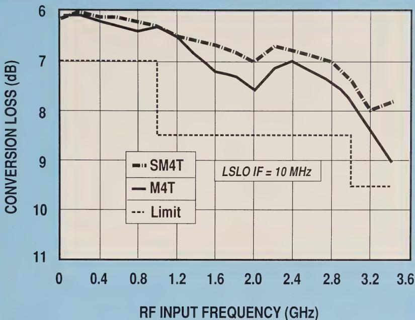
Figure 11. Electrical performance comparison of the M4T mixer in the flat-pack and SMFLAT packages.
