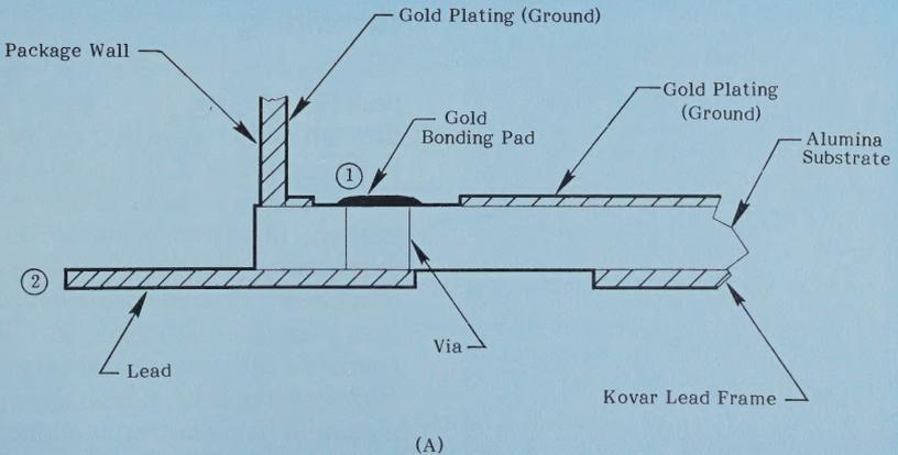
**Figure 3A.** A cross-section of the SMT-8 package showing the leadframe, ceramic base, metal via and kovar wall.
