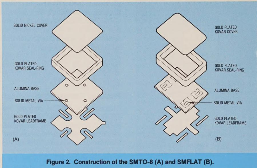
**Figure 2. Construction of the SMT0-8 (A) and SMFLAT (B).**
