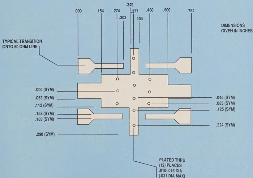
Figure 5B. Printed-wiring-board layout for the SMFLAT: 12-hole configuration.
