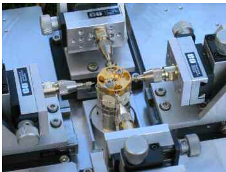
Fig. 10 Fixture to position the YIG spheres exactly in the center of the coupling loops inside the filter body
