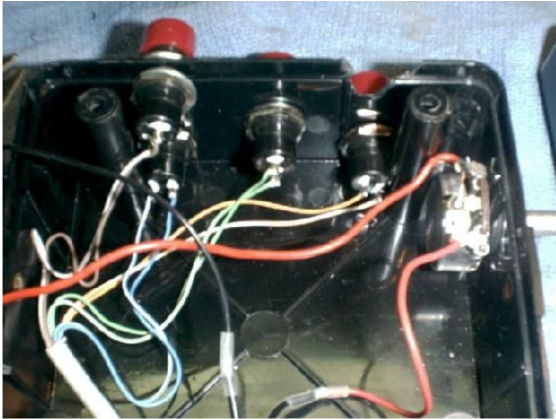
Close-up internal view of the speaker. The big RED wire is the speaker's positive (+) lead.
