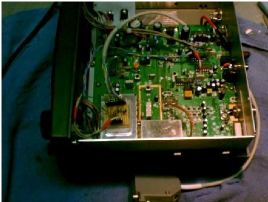
Internal view of the PRO-2042 scanner. The resistor/diode interface network is on the lower left. It routes, via SIP sockets, to a female DB-25 connector coming out the back of the scanner.
