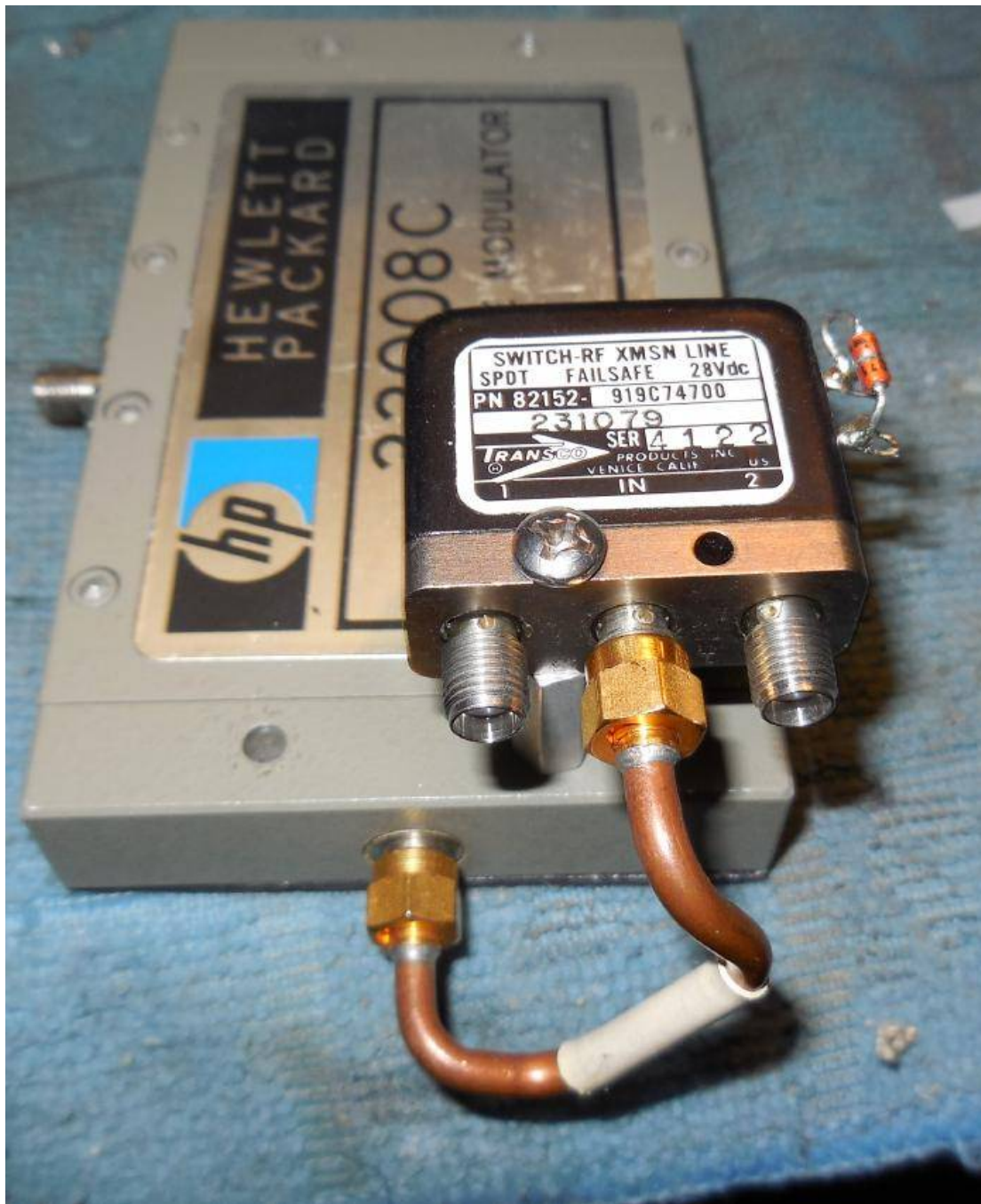
Closeup view of the HP33008C PIN modulator and the Transco 82152–919C74700 SPDT RF relay used for selecting the transmitter output port.
