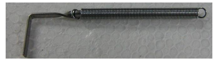
Push a small-diameter spring onto the shortened tension wrench handle. The spring used for this particular wrench is 2-inches long with a 3/16-inch inside diameter. It fits the wrench perfectly. You'll want to purchase a vast assortment of different spring lengths and spring tensions to experiment with.
