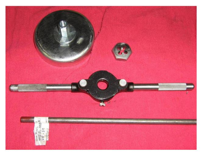
Next, get a six inch long piece of 5/16–inch diameter steel rod and a 5/16–18 thread die. You'll need to thread one end of the steel rod to screw inside the coupling nut.
