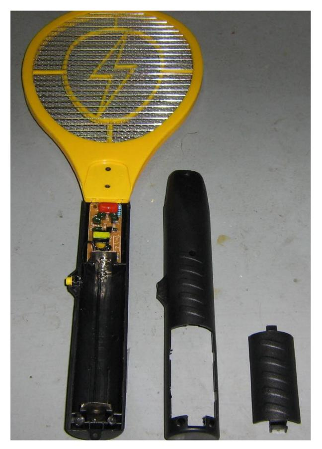
Taking the electronic insect zapper apart. It runs from two "D" size batteries. It says it generates 1,500 VDC, but its output will vary with the load under test.
