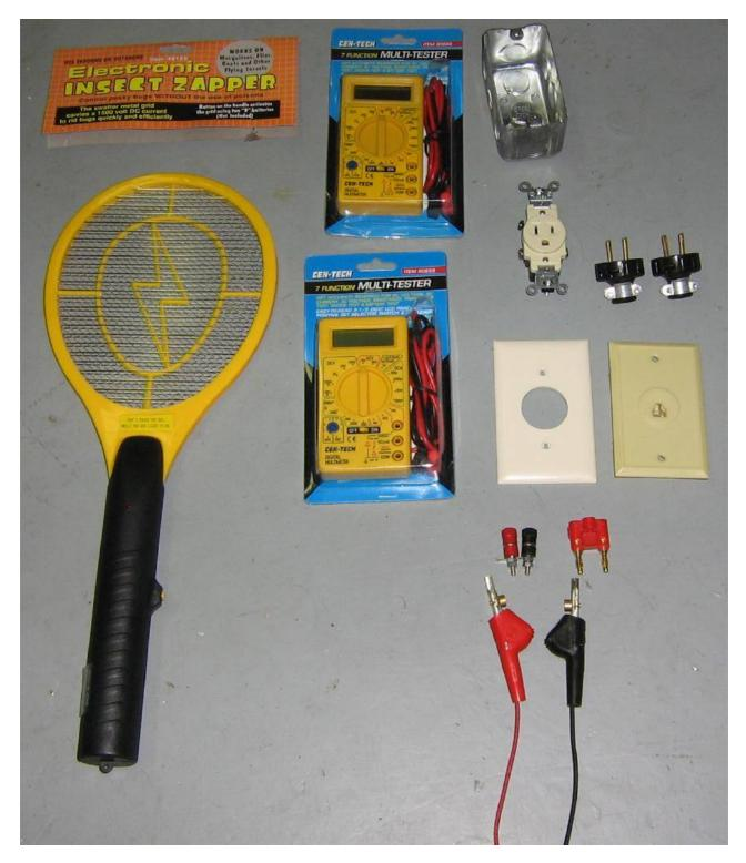
Components you'll need. The source for the high–voltage power supply will come from a Harbor Freight Tools Electronic Insect Zapper (#40122). The two Cen–Tech multimeters are also from Harbor Freight Tools (#90899). To the right of the meters are the parts needed for the outlet and also banana jacks for connecting a pair of J.S. Popper clips. A wall mounted RJ–11 telephone jack is shown to the right of the outlet plate.
