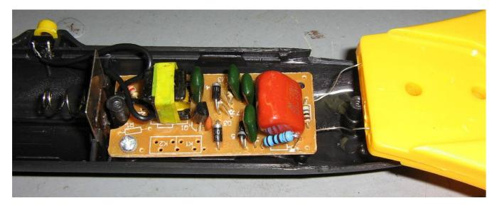
High-voltage power supply mounted inside the electronic insect zapper. Be careful to note the wiring when you remove it.
