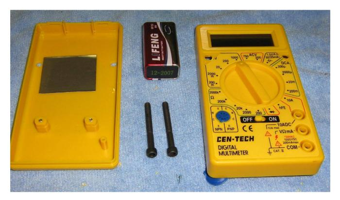
Preparing the digital multimeters. Two 3/16–inch holes are drilled through both plastic covers. They will be mounted to the case using two 1.5–inch long #8 screws and locking hardware. They'll need to be removable to replace the internal 9 volt batteries.
