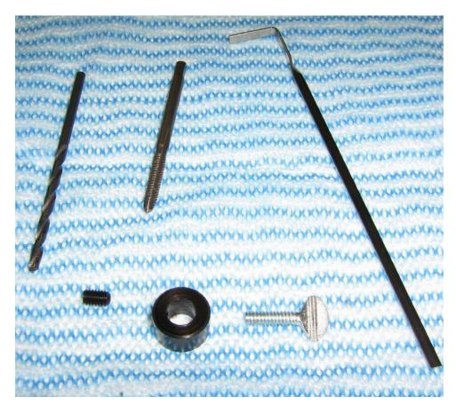
Tools needed. You'll need a #6–32 tap and #36 drill bit for the thumbscrew. Drill and tap on the opposite side of the stock set screw.
