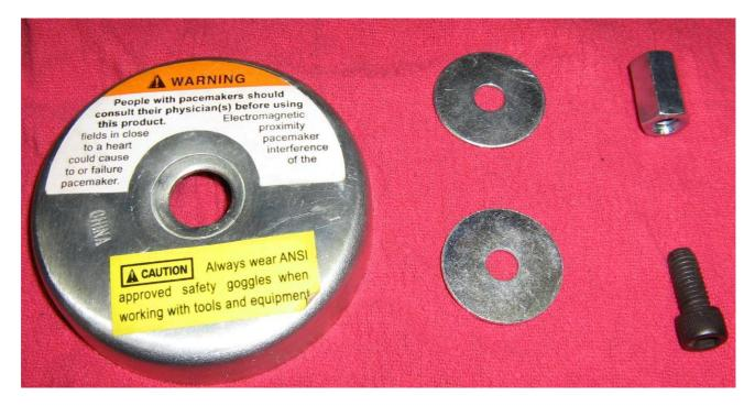
Then get two 1.25–inch outside diameter (5/16–inch inside diameter) fender washers, a 5/16–inch coupling nut, and an inch long 5/16 bolt.
