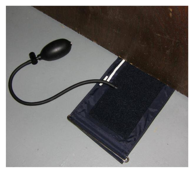
To use it, slide it underneath the door to be lifted. It should be located *away* from the hinge side for maximum "upwards" pressure on the door.
