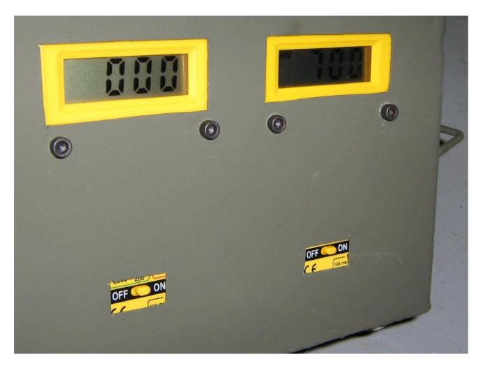
Main power is on. Meter close up picture. The meter on the left is reading the current draw (none) and the meter on the right is reading the high–voltage output (700 volts).
