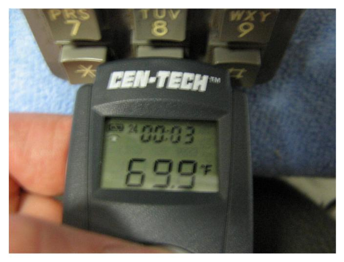
Testing. The Non–Contact Infrared Thermometer is held against a key to measure its ambient temperature, 69.9°F in this case.
