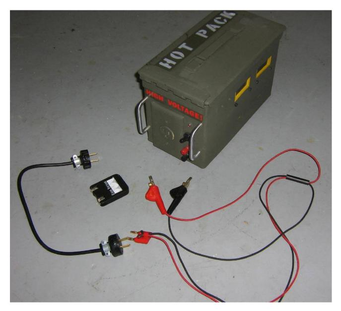
Accessory overview. A small AC plug-to-plug adapter is shown on the lower-left, the black square thing is a retractable RJ-11 phone extesion, and finally a set of J.S. Popper clips connected to a dual-banana plug.
