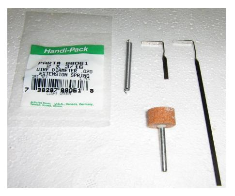
Feather tension wrench parts overview. A stock Southern Ordnance, Long Twist–Flex (TW–03) tension wrench is shown on the far–right. Cut the handle down so it is approximately one inch long. Use a Dremel tool with a cut–off wheel attachment, then debur the cut end with an abrasive wheel attachment.
