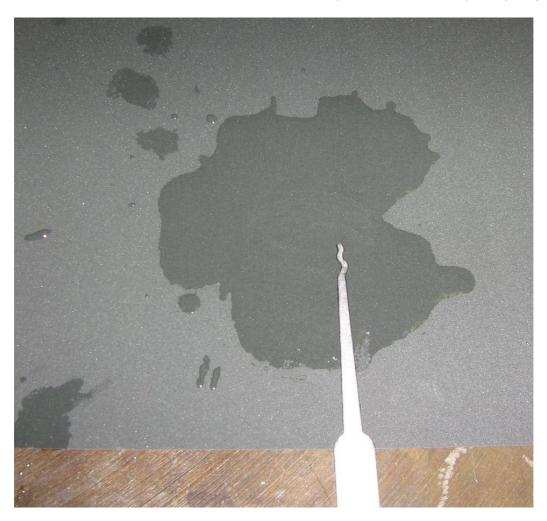
Lightly sprinkle some water onto the 1000 grit sandpaper. Work the lock pick over the sandpaper in a figure–eight pattern being sure to rotate the pick from time–to–time to get both sides. The idea is to remove any "high" spots on the pick's sides while smoothing down the edges.
