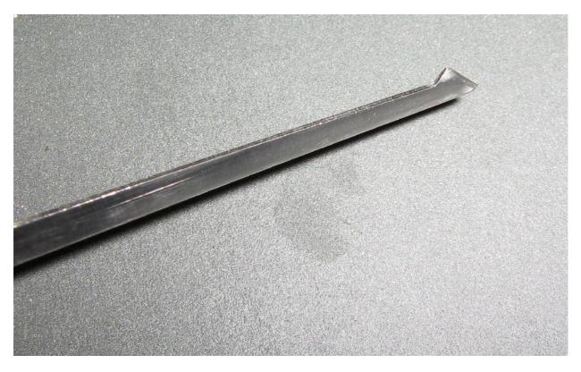
Picture showing some of the high spots being removed from the lock pick. Note the sanded areas near the tip of the lock pick.
