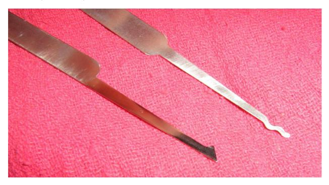
After the pick has been sanded, you can then perform the final step of polishing the pick to a mirror–like finish. Apply some polishing compound to the buffing wheel in the Dremel tool and lightly work both sides of the lock pick.
