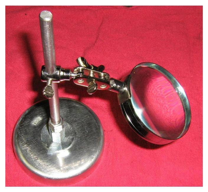
Screw the steel rod into the magnetic base and slide the magnifying glass attachment onto the rod. Lock it into place with the thumbscrew.
