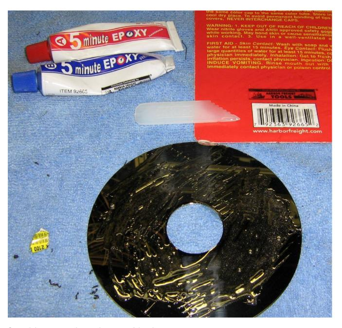
Spread the epoxy resin out along one of the platters.
