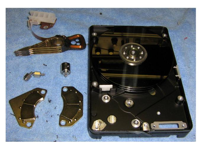
Remove the rest of the mechanical pieces. The magnets on the lower–left are very powerful and can be useful in other projects.
