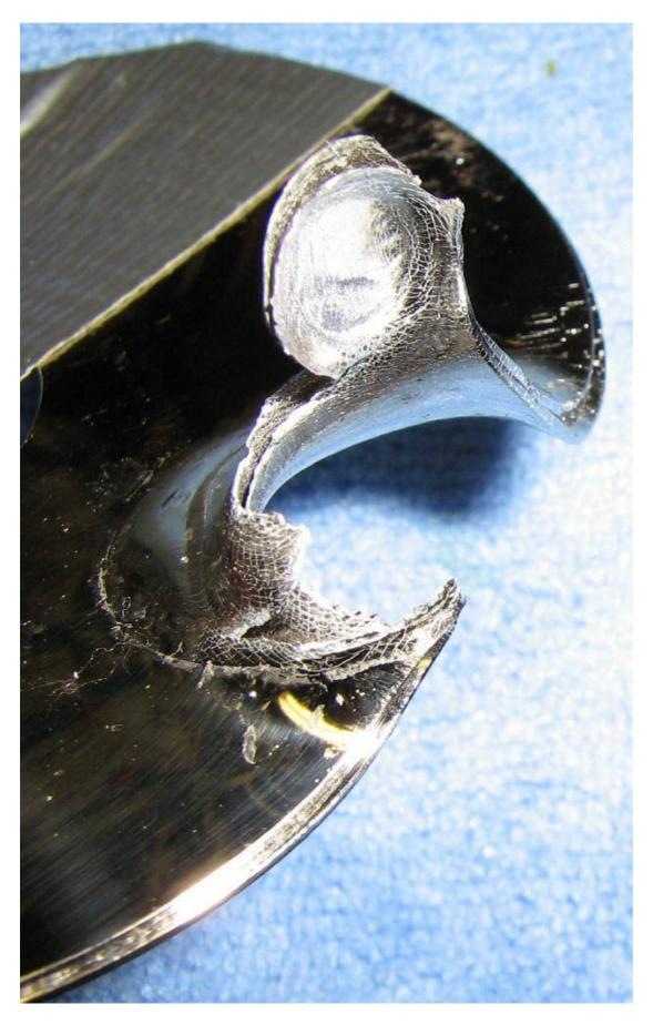
Dual hard drive platters epoxied together – .45 Colt exit.
