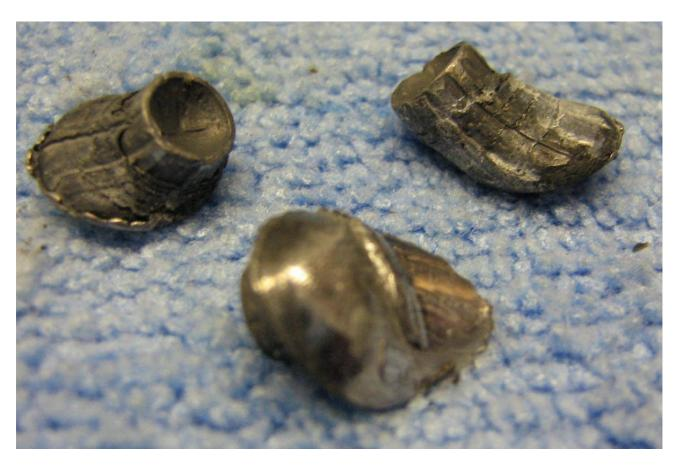
The heavy leather gloves and dual hard drive platter combination could catch the .22 LR bullets.
