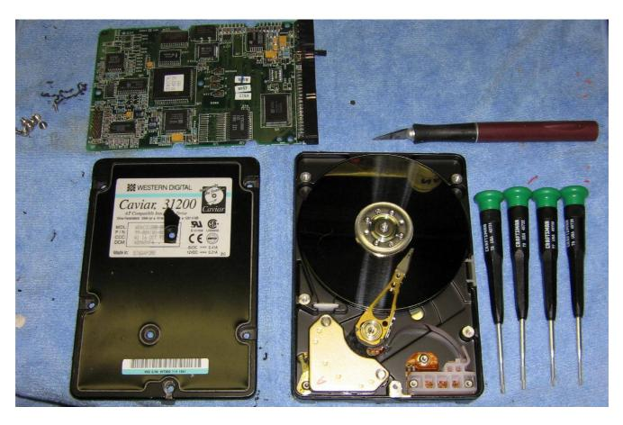
Take the hard drives apart using Torx screwdrivers and an X-acto knife. Save the controller PC board as it is a good source of surface mount components.
