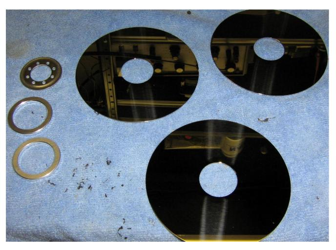
Then remove the individual platters. There are usually two or three platters in each hard drive.
