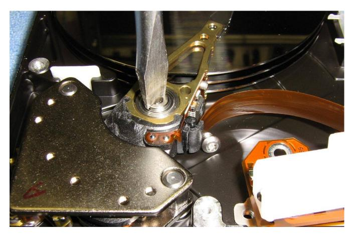
Remove the armature for the drive's magnetic head using a regular screwdriver as shown above.
