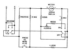
Fig. 2—KS-8455 Test Set (Schematic Diagram)
