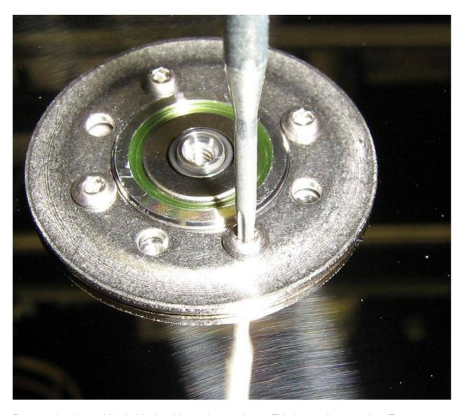
Remove the plate which holds the drive's platters down. This is usually a small #6 Torx screw.
