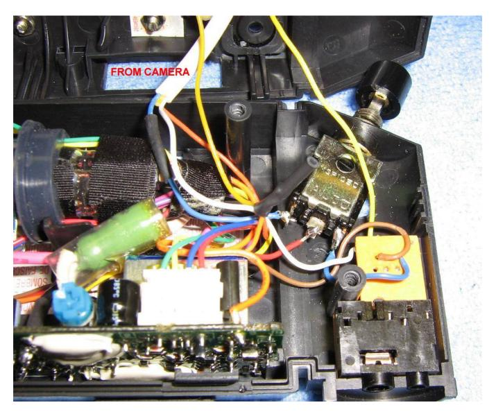
Wires resolder in. The **RED** wire on the center terminal of the SPDT switch is the viewer's main video input. The **BLUE** wire on the right is from the 1/8–inch external video input jack, and the *other* **BLUE** wire (left side) is the video input from the CMOS night vision camera.
