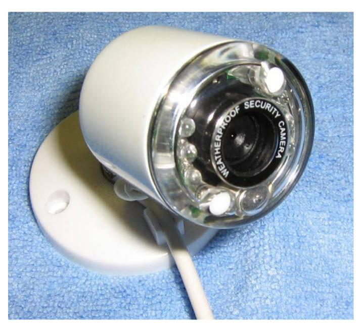
Closeup of the video camera. It is completely sealed inside a fairly weatherproof package. Six infrared LEDs are used for illumination when operating in the dark. The addition of more infrared LEDs with some type of focusing system will greatly increase the "night vision" performance of the camera.
