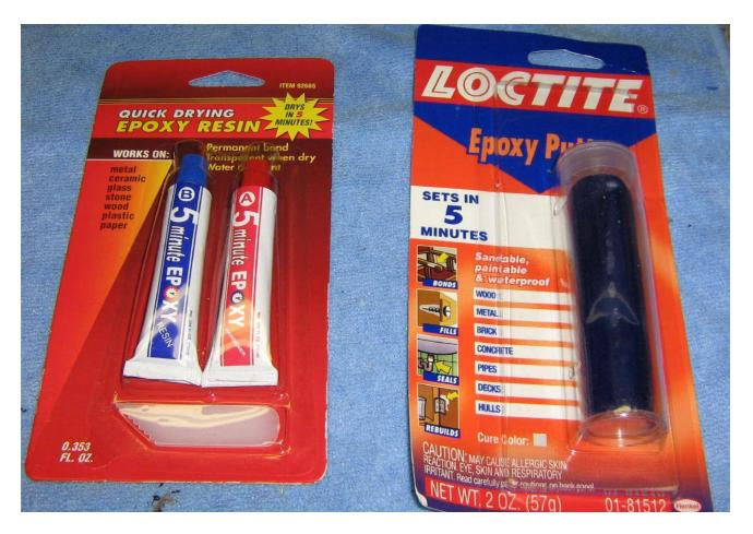
Some of the two-part epoxy resins and putties used for this test. Use the epoxy resin (left) to sandwich two disk platters together for greater strength, then use the epoxy putty to hold the improvised armor in the location you need.
