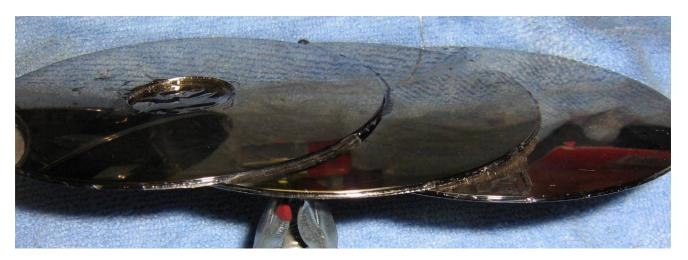
Here are three sandwiched dual-platters epoxied together. Each one overlaps, covering the center hole on the platters underneath it.
