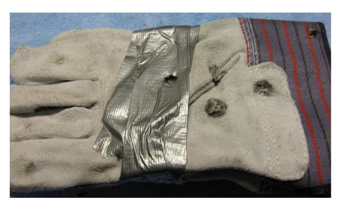
A different test with the dual hard drive platters behind a pair of heavy leather gloves – .45 Colt went straight through. The idea is that thick leather can be used to reduce or even prevent any flesh burns from IEDs.
