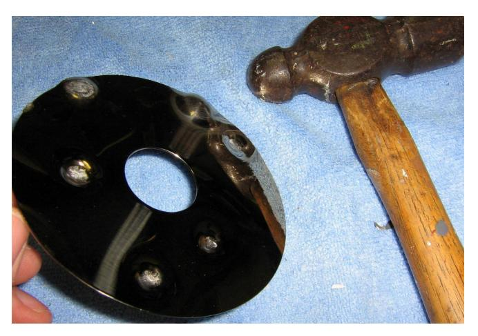
Initial strength test using a ball peen hammer. The individual drive platters appear to be very light (0.5 oz) aluminum discs with some sort of coating. Maybe it's the coating that gives them strength?
