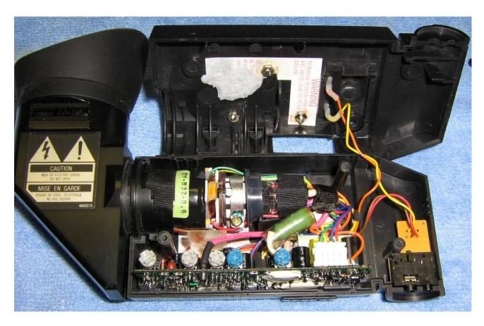
Inside the "stock" **Portable Video Camera Viewer** as we left it. External video input is on the lower-right.
