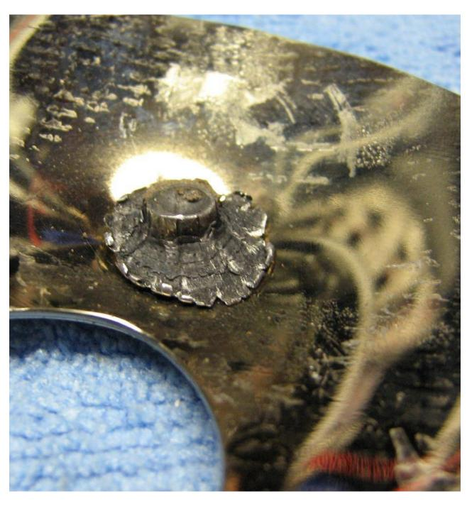
A different set of dual hard drive platters epoxied together – .22 LR with the same results.
