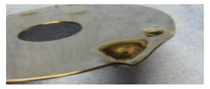
Close up of a hammer hit on a single disk platter.
