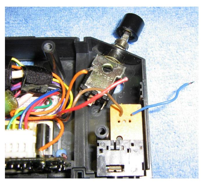
Find a convenient location and install a SPDT switch. This will select between which video input is sent to the viewer's display. The external video input still comes in via the 1/8–inch panel jack and is soldered to the other pole on the input selector switch.
