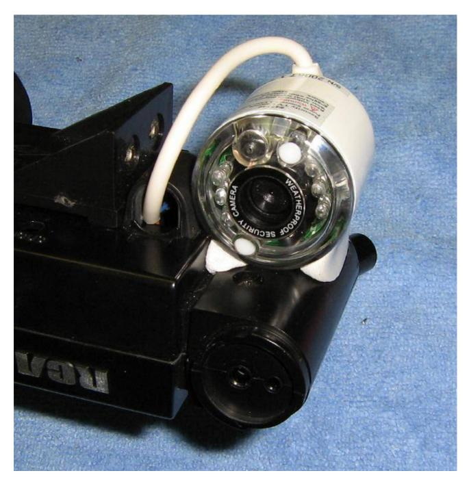
Epoxy the camera to a suitable location on the outside of the **Portable Video Camera Viewer**. Be sure it is pointed in the right direction and "right-side" up – test this ahead of time! Also be sure no screws or adjustment holes are covered up.
