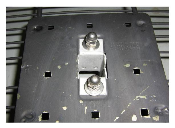
The only modification to the stock parabolic reflector is to the feed's mounting brackets. Since we'll be making a new feed arm, the original brackets should be drilled out (they are rivoted) and replaced with 1/4-inch stainless steel hardware. This helps to distribute the added weight of the magnetron mounted to the feed arm.
