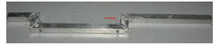
New feed arm made from 1-inch square aluminum tubing. The second little strut should have been 2-inches long, instead of only 1-inch, to help center the magnetron's horn antenna at the focal point. The aluminum feed arm was also an experiment using those "weld with aluminum" sticks you can buy at the hardware store. They say you can use only propane, but in reality, you'll need to use MAPP & oxygen to get a good "weld."
