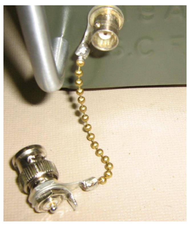
On the BNC input jack, a small chain (from a lamp pull), two solder tabs, and a male BNC connector, were used to make a protective cap which also doubles as clip—on points for alligator clips.
