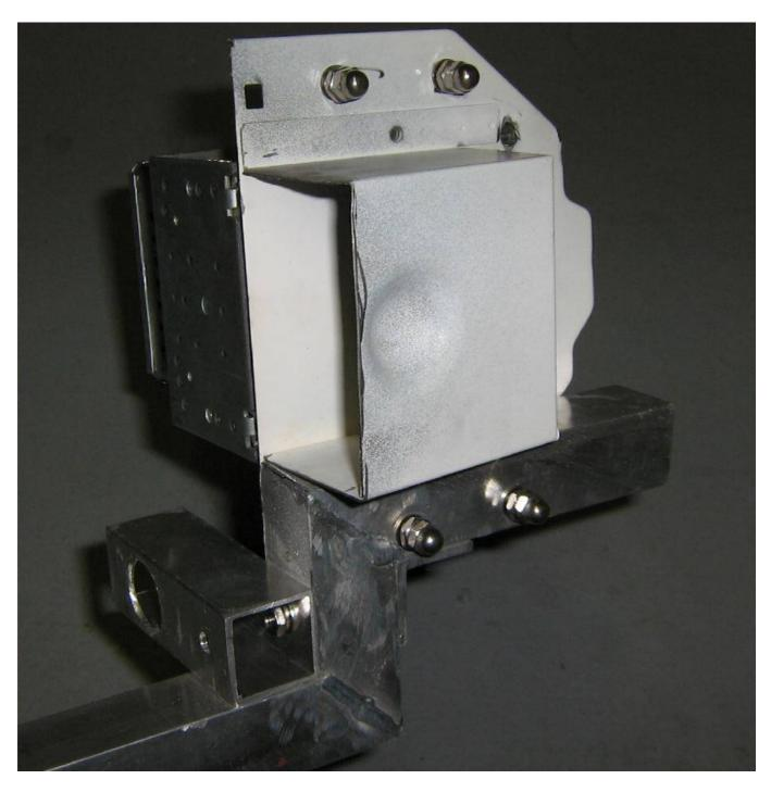
Test setup view showing the feed horn assembly for the magnetron. Refer to the **GBPPR HERF Device** project in issue #29 for more information on how to salvage the feed horn from an old microwave oven.
