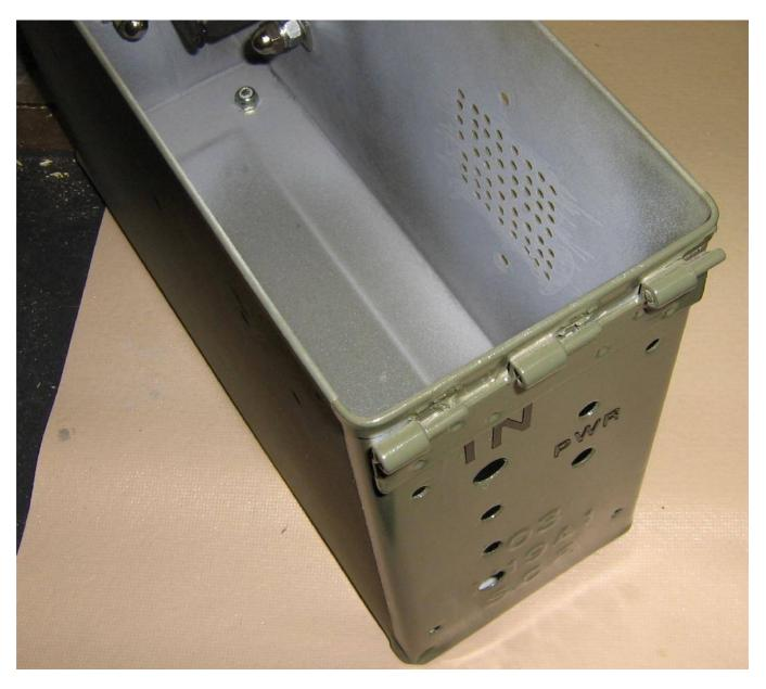
Alternate view showing the front–panel and the array of 1/8–inch diameter speaker holes. In the rear, two L–brackets secure the battery pack to the side of the case. The holes on the left side of the front–panel are for a 1/4–inch jack, a 1/8–inch jack, a RCA jack, and a BNC jack.
