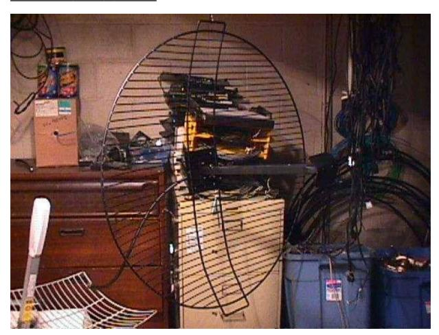
Parabolic antenna reflector used for this project. It's a Lance Industries Model 2536. This 36-inch diameter dish was originally designed for the 2.5-2.7 GHz MMDS band. The gain is approximately 26 dBi and the 3 dB beamwidth is 10 degrees. The focal length is 18-inches.
