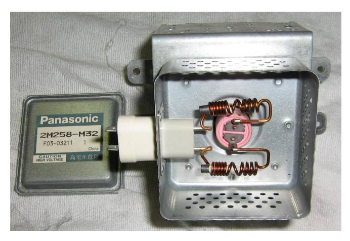
Inside the filament/cathode filter box on a Panasonic 2M258 magnetron. The large white plastic insulator is a feed–through capacitor and the two inductors keep the 2.45 GHz signal from flowing back into the filament/cathode leads. These should probably be bypassed for this application.
