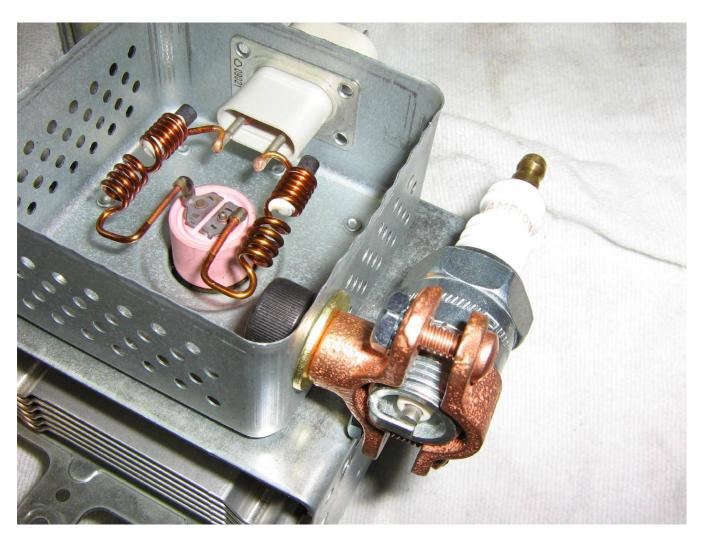
The spark plug is mounted to the magnetron by drilling a hole in the filter box and bolting it to the side. The mounting bolt is 3/8-inch, with brass washers to isolate the copper clamp. Kep nuts were also added to the ground clamp's screws to help secure the spark plug. The spark plug's gap is set to around 0.04-inches, or to fire at around 4,500 volts.
