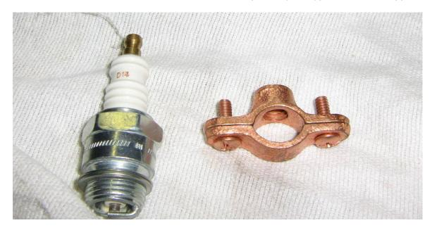
An automotive spark plug will be used for the spark gap. A Champion D14 is shown here. Be sure it *doesn't* have an internal resistor. A copper pipe ground clamp will be used to hold the spark plug, which will then be attached to the side of the magnetron's case.
