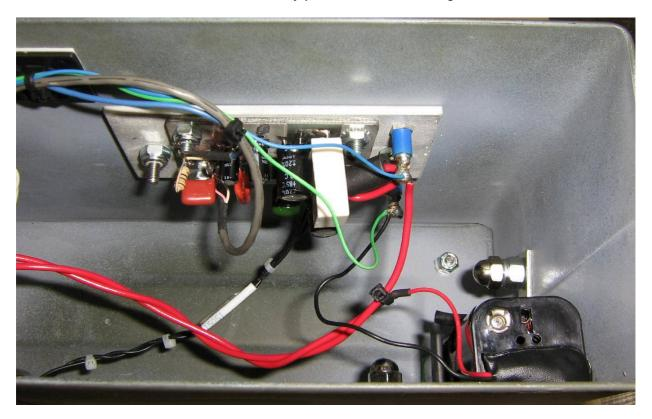
Close up picture of the main circuit board and the battery pack. Since the LM380 can draw up to one amp, you should try to use fairly heavy gauge wire for the LM380's power connections. The small blue and green wires are for the front–panel LED power indicator.
