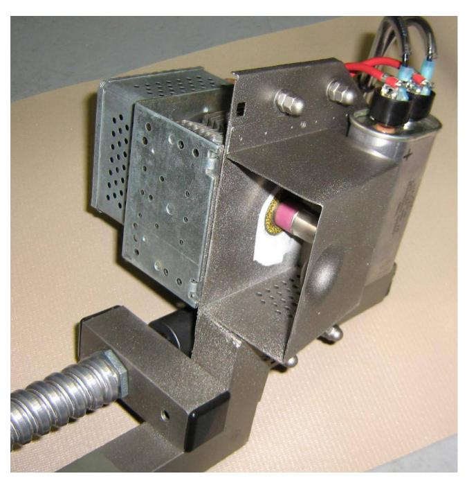
Completed feed view. The high-voltage capacitor charging line comes in via an armored cable. The high-voltage capacitor is epoxied behind the feed horn. This is only temporary, as the 1  $\mu$ F capacitor proved to be too small in value to really accomplish anything.
