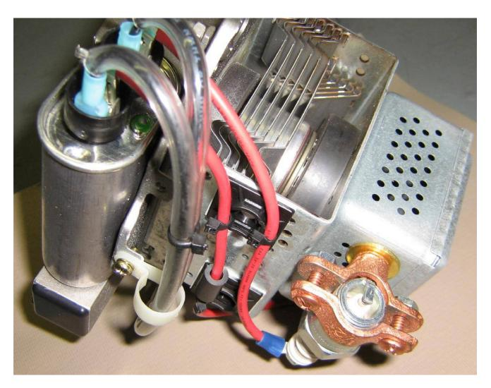
Completed top view. Note the vinyl tubing around the high-voltage charging lines. This worked out quite well. A ferrite bead was slipped around the cathode lead for good luck. Be sure all the high-voltage lines are isolated from the magnetron's case (anode). The spark plug has a handy #8 binding post if you remove the screw cap.
