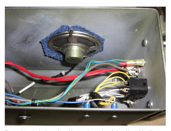
Close up picture showing the speaker and front-panel connections. A piece of "non-slip" pad is used to seal the speaker to the side of the case.
