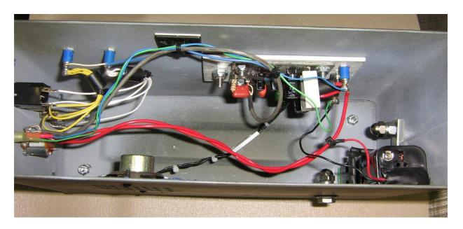
**GBPPR 1079 Audio Amplifier** internal overview. Front–panel is on the left. The common inputs and grounds from all the front input jacks tie to signal points, with an additional ferrite bead slipped over them to block any RF interference. The speaker and the main amplifier circuit board are mounted in the middle, and the "AA" battery pack is on the lower right.
