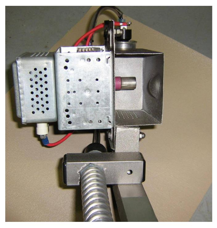
Completed view, looking down the feed horn. The microwaves are emitted from the pink ceramic probe, with the "cap" acting as a capacitor tuning hat.
