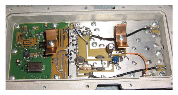
Install the new PC board, being sure it is both mechanically and electrical stable.
