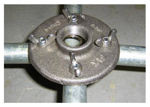
Temporarily attach the legs to the center floor stand to check everything out. You can use whatever hardware is most convenient, but wing nuts are handy for quick assembly and disassembly.
