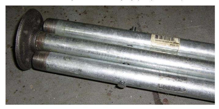
To store the mast sections during transport, drill holes through each of the 3/4-inch pipes near each end. Place a large 1/4-inch threaded bolt through them and secure with wing nuts.
