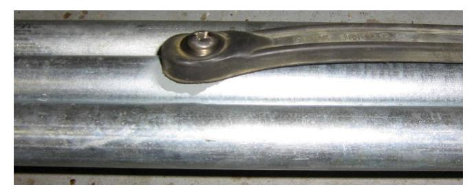
Add an optional bungee cord handle to the center mast section to make the mast bundle easier to carry.
