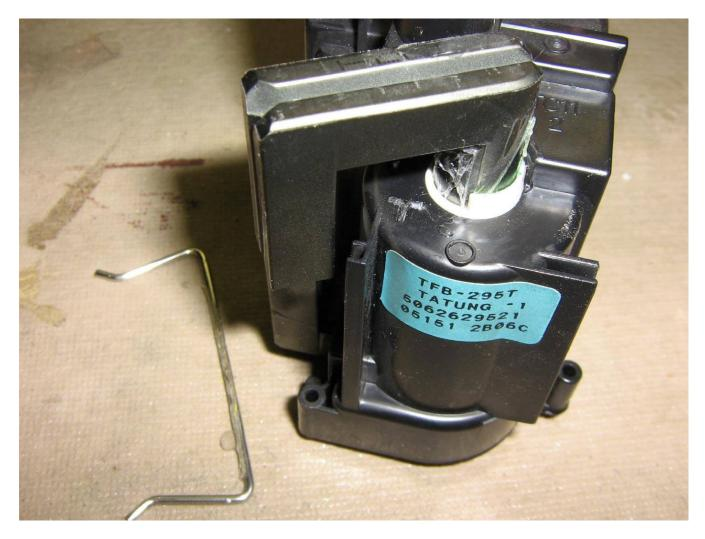
The ferrite core is split into two pieces and may be glued into place.
