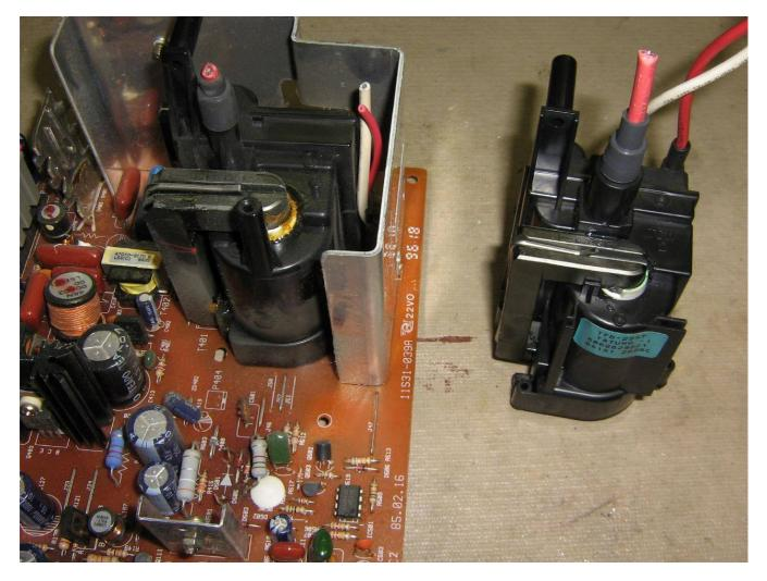
The high–voltage "flyback" switching power supply section in an old CRT–based computer monitor.
