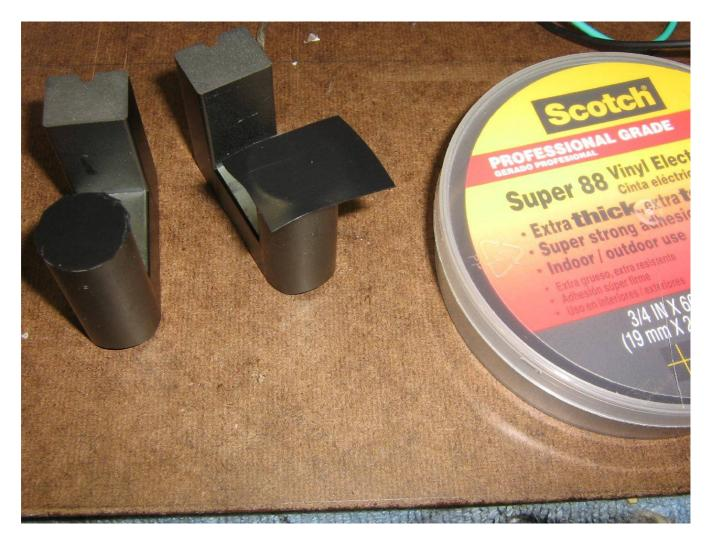
In order to keep the ferrite core from saturating, you can add a small air gap to <u>one</u> of the core's legs.
