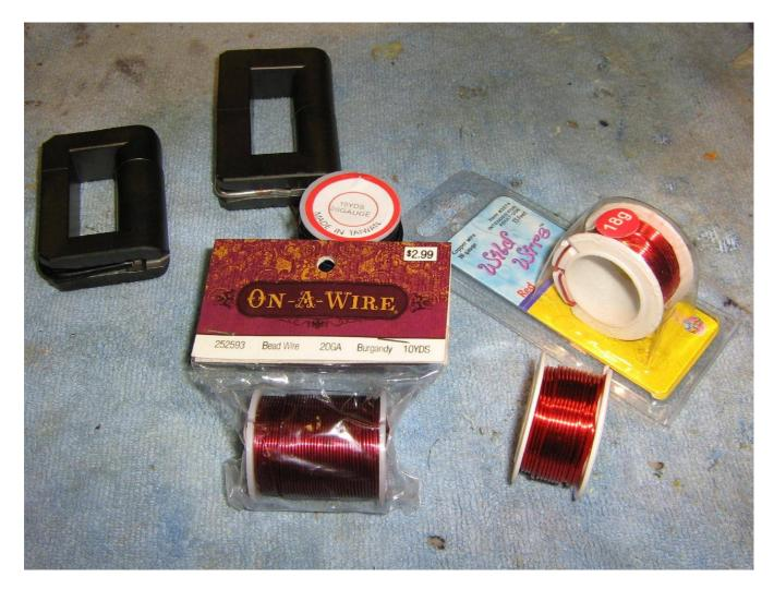
The enameled wire we'll be using and some example ferrite cores on the upper-left.
