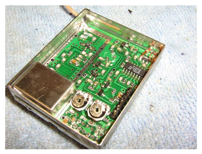
Alternate internal view of the 2.4 GHz video receiver module.
