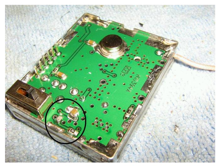
Bottom view of the 2.4 GHz video receiver module.
