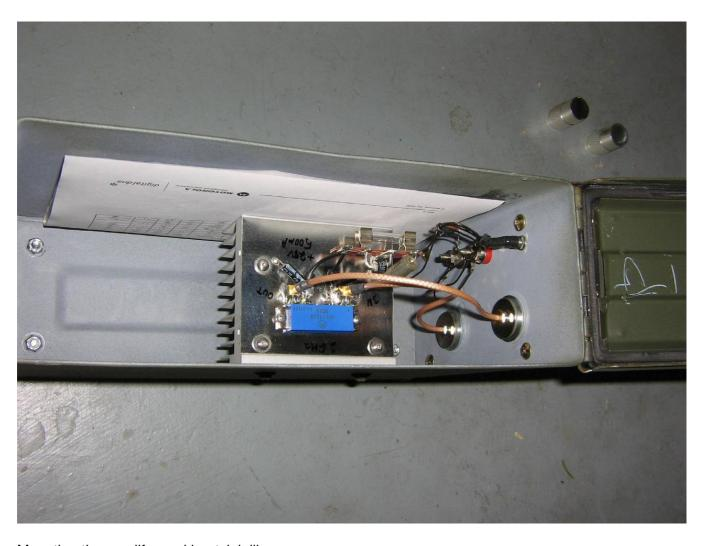
Mounting the amplifer and heatsink like so.
