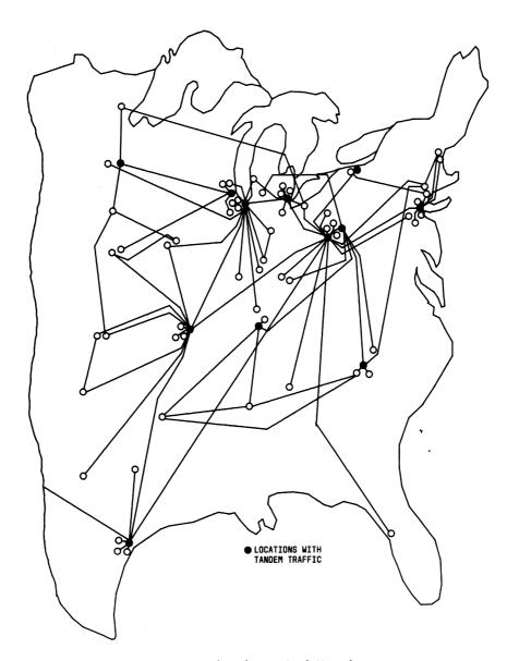
Fig. 1—Typical Tandem Tie Trunk Network
