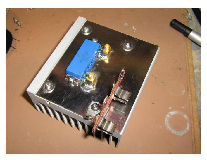
Attach the tin sheet to the heatsink using the proper hardware. Be sure the tin plate fits the heatsink and that there are no air gaps.
