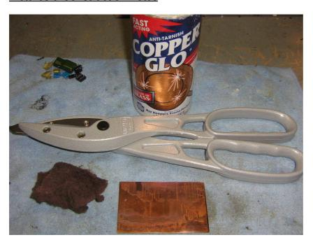
Use a Midwest M1200 3.5-inch snips to cut the PC board to the size you require. These are very nice snips which cost only around \$30. Harbor Freight Tools makes a knock-off for \$10, but the final cut will not be as precise.
