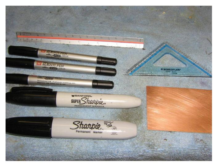
Shown above are some of the markers used for the laying out the etch resist pattern. The main layout is done using a Sakura IDenti-Pen which has a dual tip for fine and extra fine lines. These Sakura pens are available at Michaels hobby stores.
