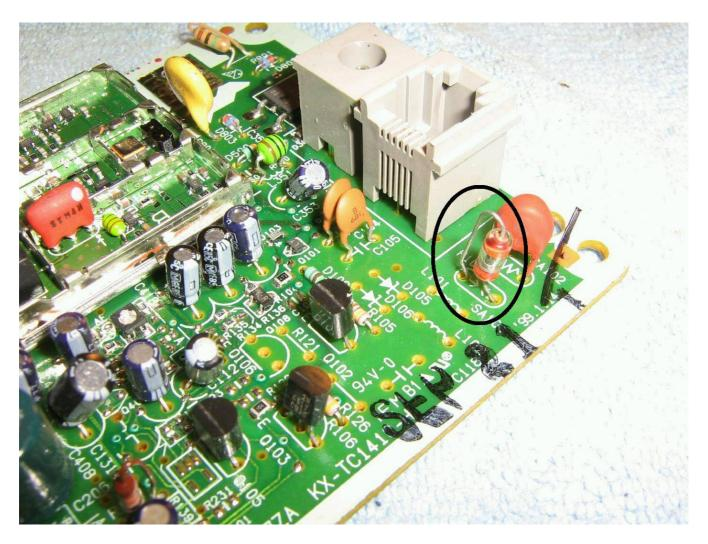
For additional circuit protection, an optional spark gap can be added across the primary of the transformer. The spark gap provides "front line" defense against any high voltage spikes being coupled into the transformer.
