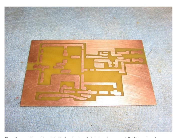
Clean the remaining etch resist off using denatured alcohol and a non-metallic 3M scrub pad.
