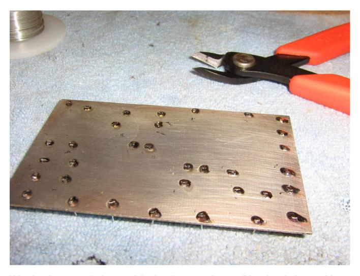
Using the wire cutters, trim the ground via wires down at much as possible *only* on the bottom of the PC board.
