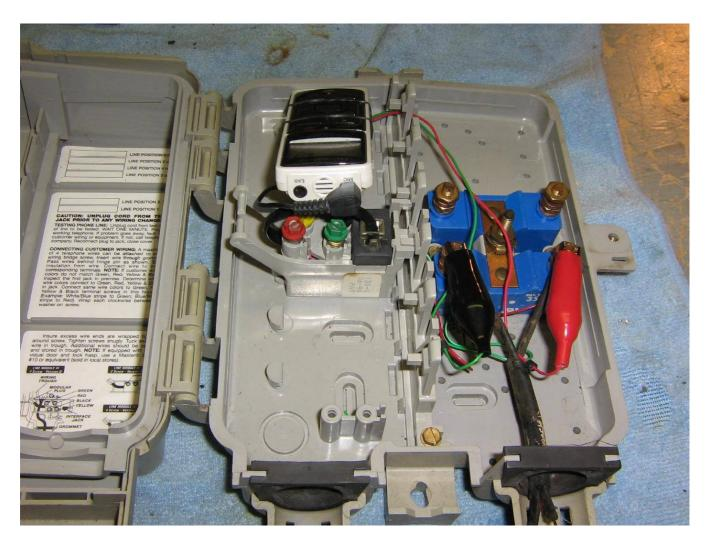
If you have access to the proper "tamper–proof hex" security bit, you can install the tap in the "Tel. Co. Access Only" side of the network interface box.
