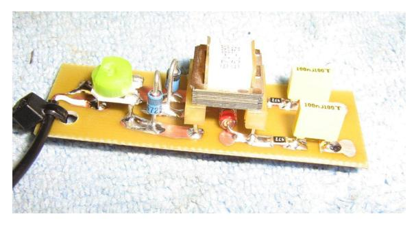
Close up view of the telephone audio interface board.
