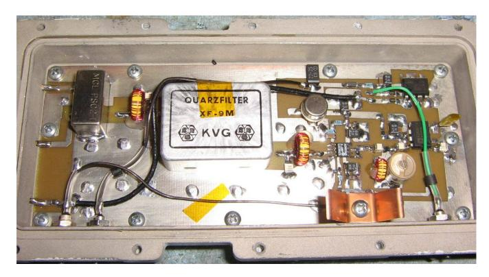
Overview of the 9 MHz resolution filter, 9 MHz final IF amplifier, and the logarithmic detector.
