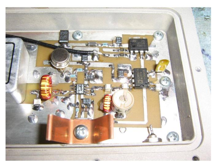
Closeup view of the Analog Devices AD603 and AD8307. The RSSI DC voltage output from the AD8307 is buffered by a LM358 op–amp.
