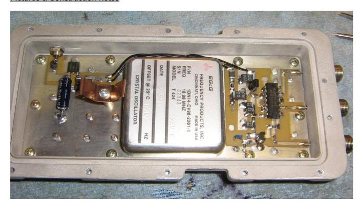
10 MHz Temperature Compensated Crystal Oscillator (TCXO) time base.
