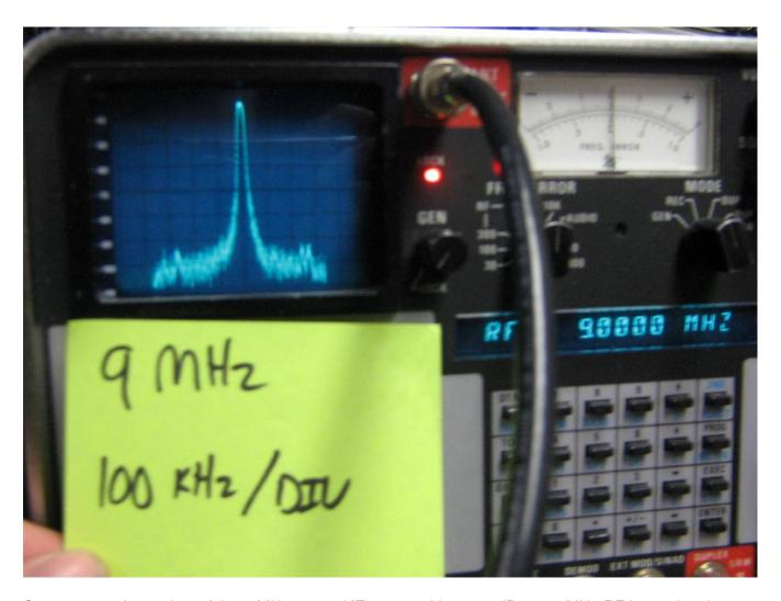
Spectrum analyzer view of the 9 MHz second IF output with a –30 dBm 436 MHz RF input signal.
