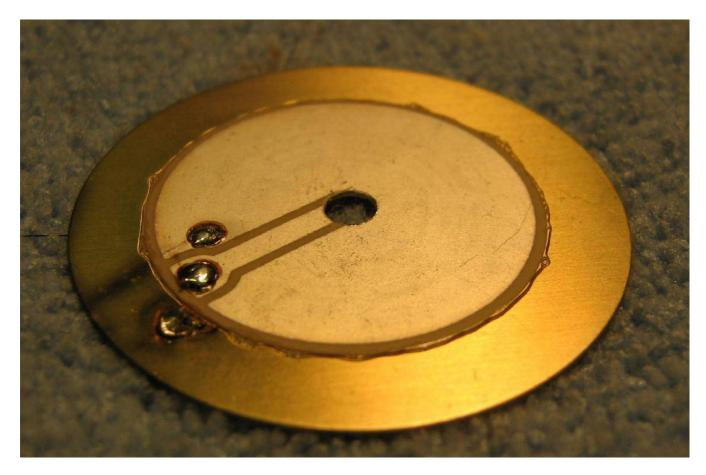
Drill or punch a 1/8-inch hole in the center of a piezoelectric buzzer element.
