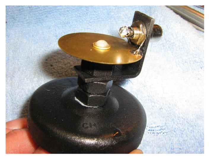
Completed magnetic-mount contact microphone.
