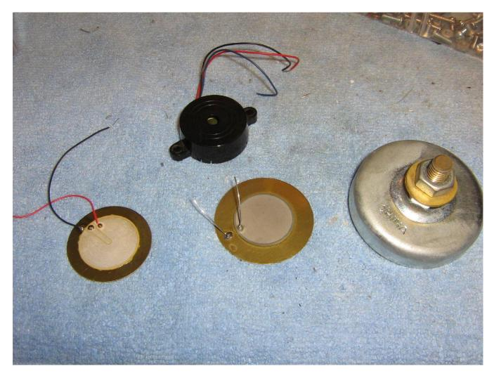
Example of some piezoelectric elements from old buzzers.
