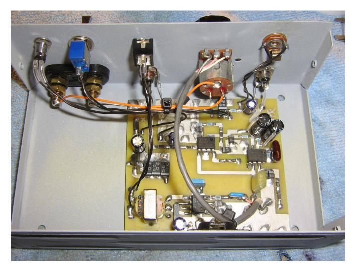
Mounting the circuit board inside an old printer switch case.
