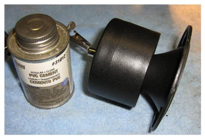
Slide the piezo horn tweeter into the 2-inch cap and secure using PVC cement.
