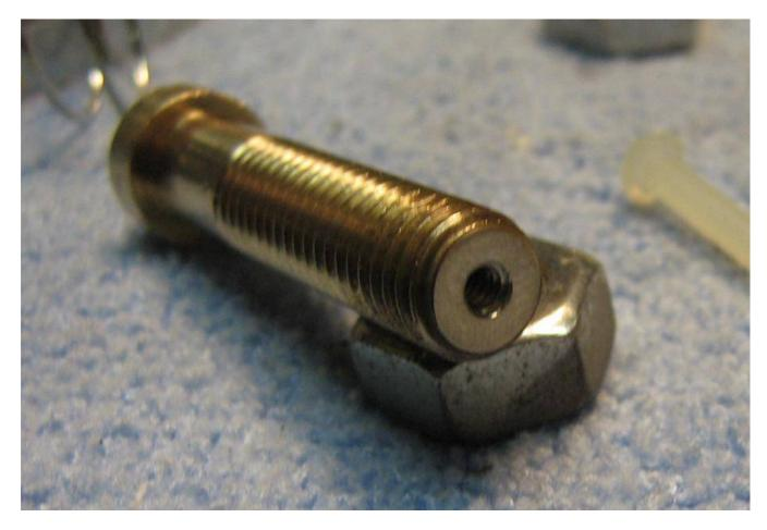
Very carefully drill and tap a #4–40 screw hole in the center of the "threaded end" of the magnetic ground block's brass stud.
