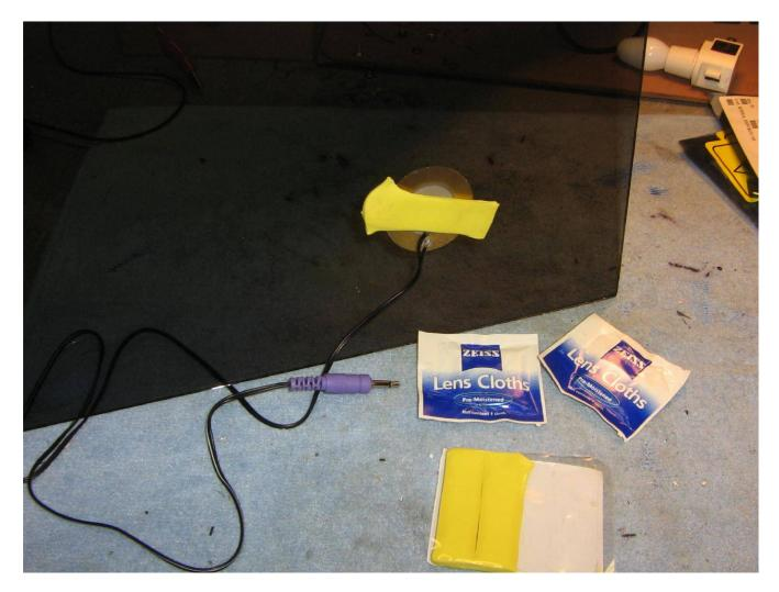
For "through a window" applications, attach the piezoelectric element directly to the target window using Elmer's Poster Tack reusable putty adhesive.
