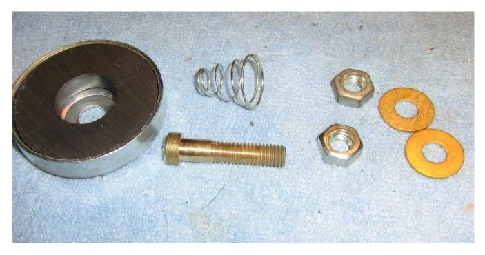
Overview showing the pieces of the magnetic ground block including the main spring-assisted brass stud.
