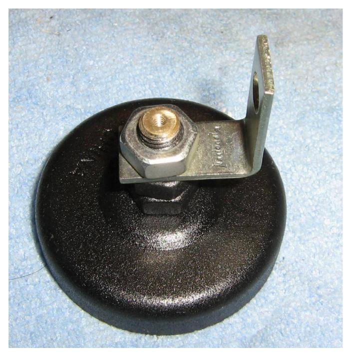
Mount a small L-bracket to the threaded brass stud of the magnetic ground block, as shown above. This will be used to hold a RCA phono jack for the output of the contact microphone.
